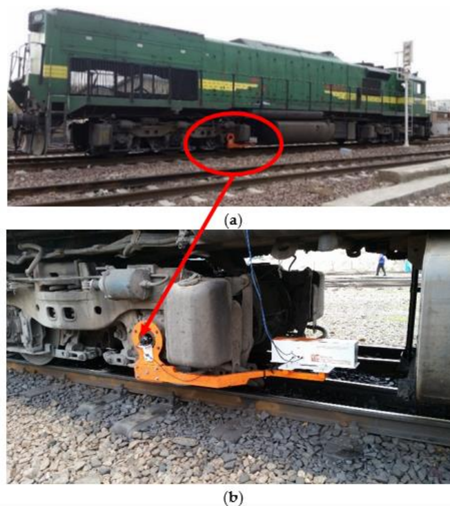
Figure 3. Data acquisition of track stiffness: (a) recording car; (b) laser/camera system installed to bogie frame.
