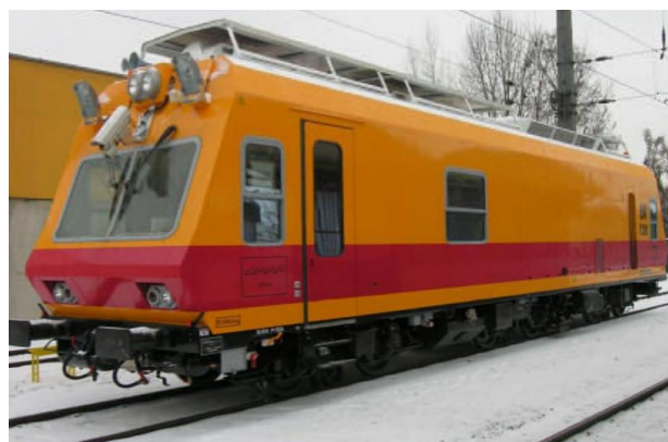
Figure 2. A view of the geometric track recording car (EM120).
