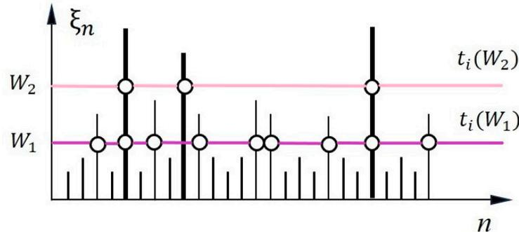
Figure 7. Graph of the random process of exceeding two critical levels of power consumption.
