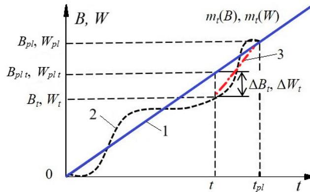
**Figure 2.** Schedule of the production plan for the output  $B$  with power consumption  $W$  for a single technological process: 1—planned schedule; 2—potential option for production output; 3—alternative option for production output in one of the stages.
