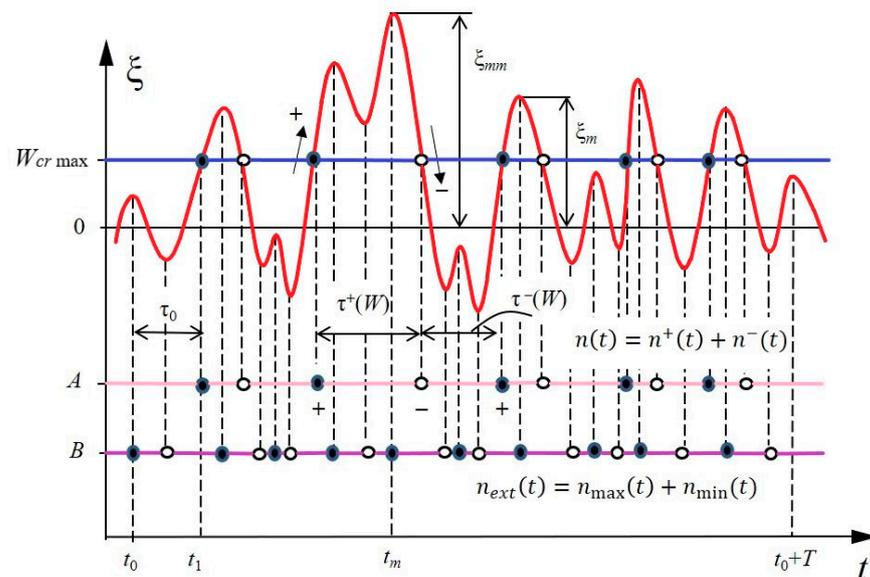
**Figure 6.** Graph of a sample realization of the random function  $\zeta(t)$  and characteristics of its trajectory level-crossings  $W(t)$ .
