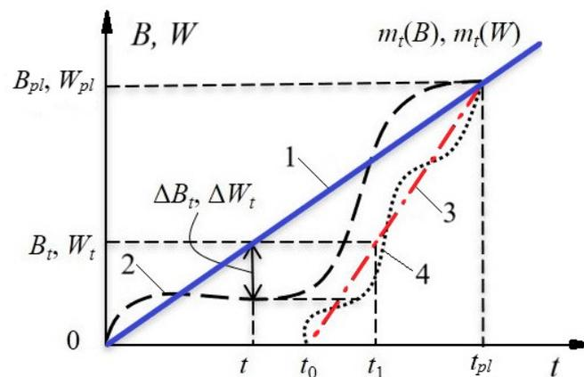
**Figure 3.** Schedule of the output plan  $B$  and electricity consumption  $W$  with a delay caused by the repair of an electrical equipment unit: 1—planned; 2—possible option for the output production; 3—option for the output production at speed  $V_{\max}$ ; 4—alternative option for the output production at speed  $V_{\max}$ .
