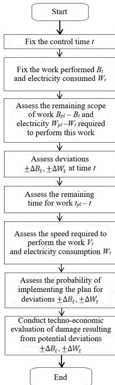
**Figure 4.** Block diagram of the algorithm for analyzing the current state of technological process and power consumption behavior.
