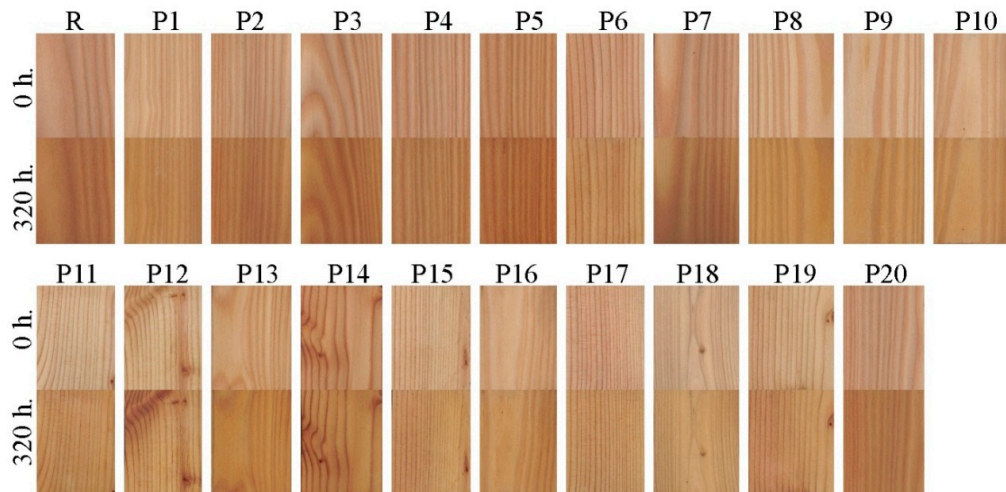
Figure 3. European larch wood with color stabilizing pretreatments (P1–P20) before and after 320 h of AA.
