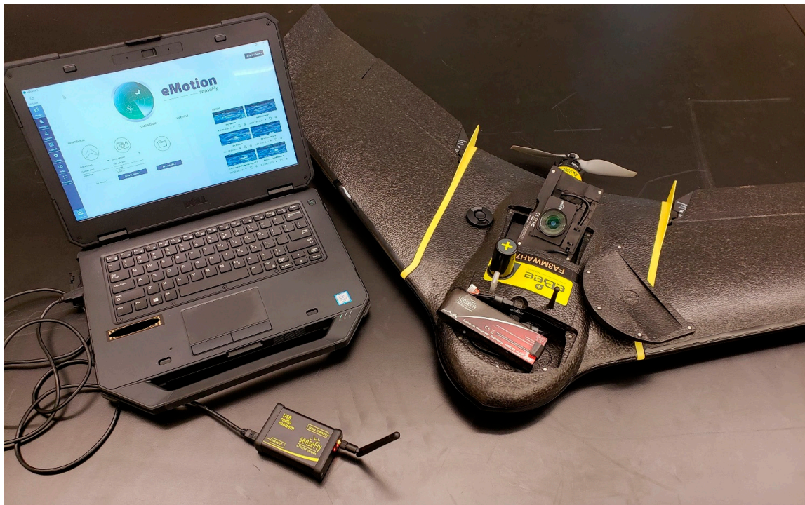
Figure 4. eBee Plus Unmanned Aerial System (UAS) with the sensor optimized for drone applications (S.O.D.A) and eMotion3 flight planning software.
