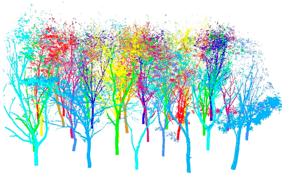
Figure 2. Individual trees extracted automatically from the point cloud data of the plot.
