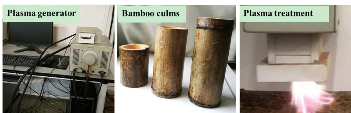
**Figure 1.** The plasma treatment of bamboo culms using a plasma generator.
