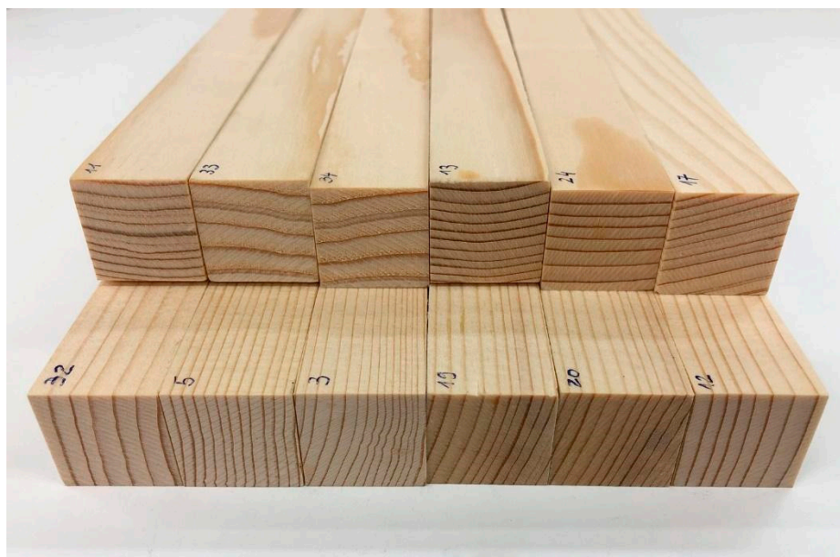
Figure 9. Photograph of the 12 tested samples, ordered by their diminishing density from left to right. Top six samples were loaded radially, while the bottom six were tested tangentially.
