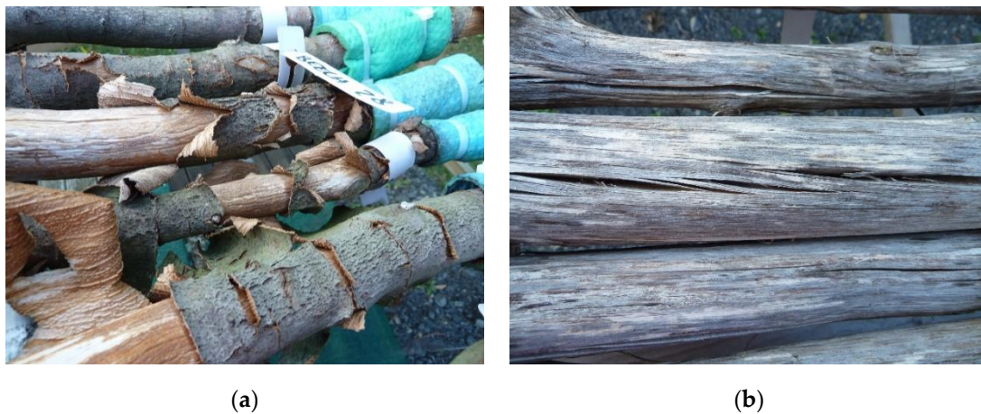
Figure 5. Visual appearance of above-ground specimens after 6 months of exposure. (a): severe flake off of bark on Beech specimens with sponge wrapping. (b): formation of cracks in Hazel specimens without bark.
