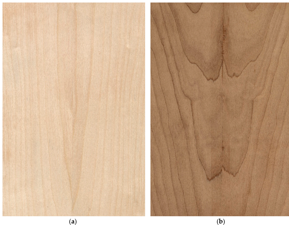
Figure 12. (a) Sample of untreated birch veneer. (b) Sample of treated veneer under a temperature of 200 °C for 2 h.
