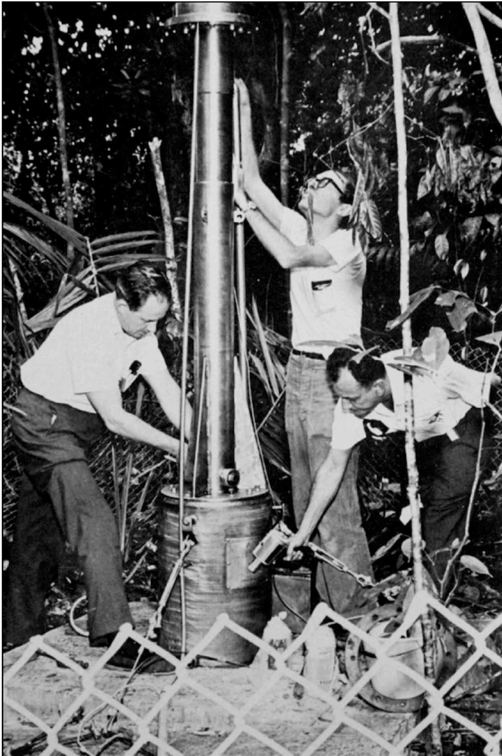
Figure 2. Scientists installing the base and casing for the Cesium radiation source in the Luquillo Experimental Forest. Photo reproduced from [53].
