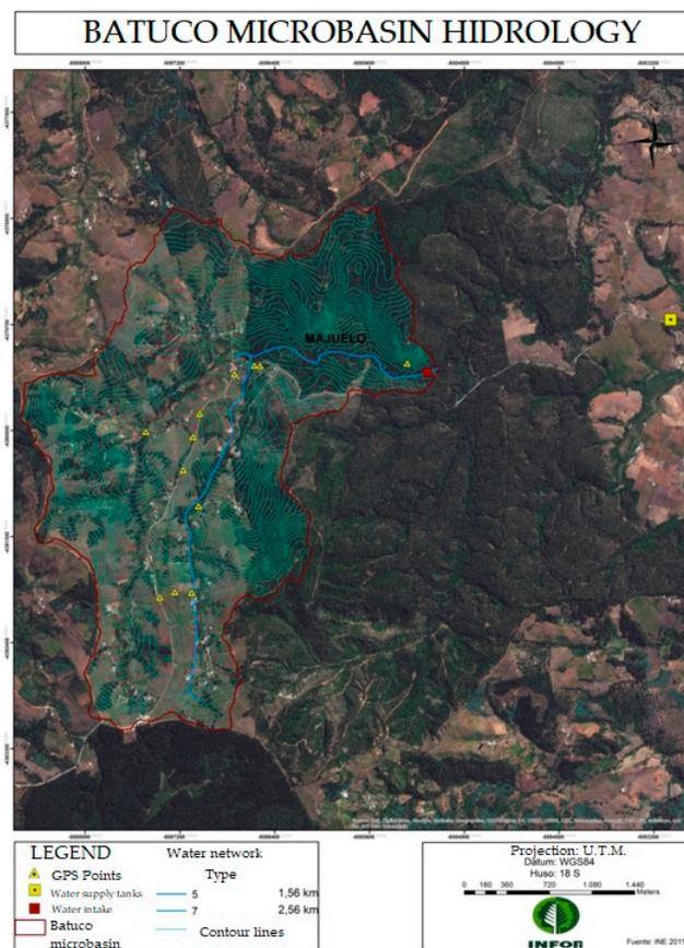
**Figure 2.** Water supply system (light blue), water intake area (red dot), and supply pumps (yellow square) of Batuco Water Committee, Global Positioning System (GPS) points (yellow triangle). Source: Compiled by authors from [www.bosquesyagua.cl](http://www.bosquesyagua.cl) and field study.
