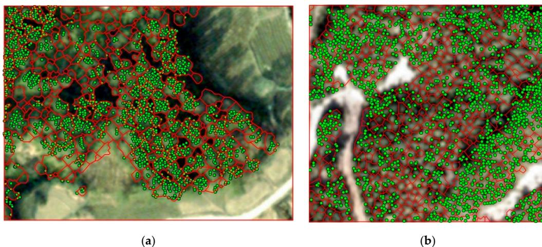
**Figure 7.** Distribution of LiDAR pulse points (green) in the tree crowns in the two test forest areas. (a) Forest plot 1. (b) Forest plot 2.
