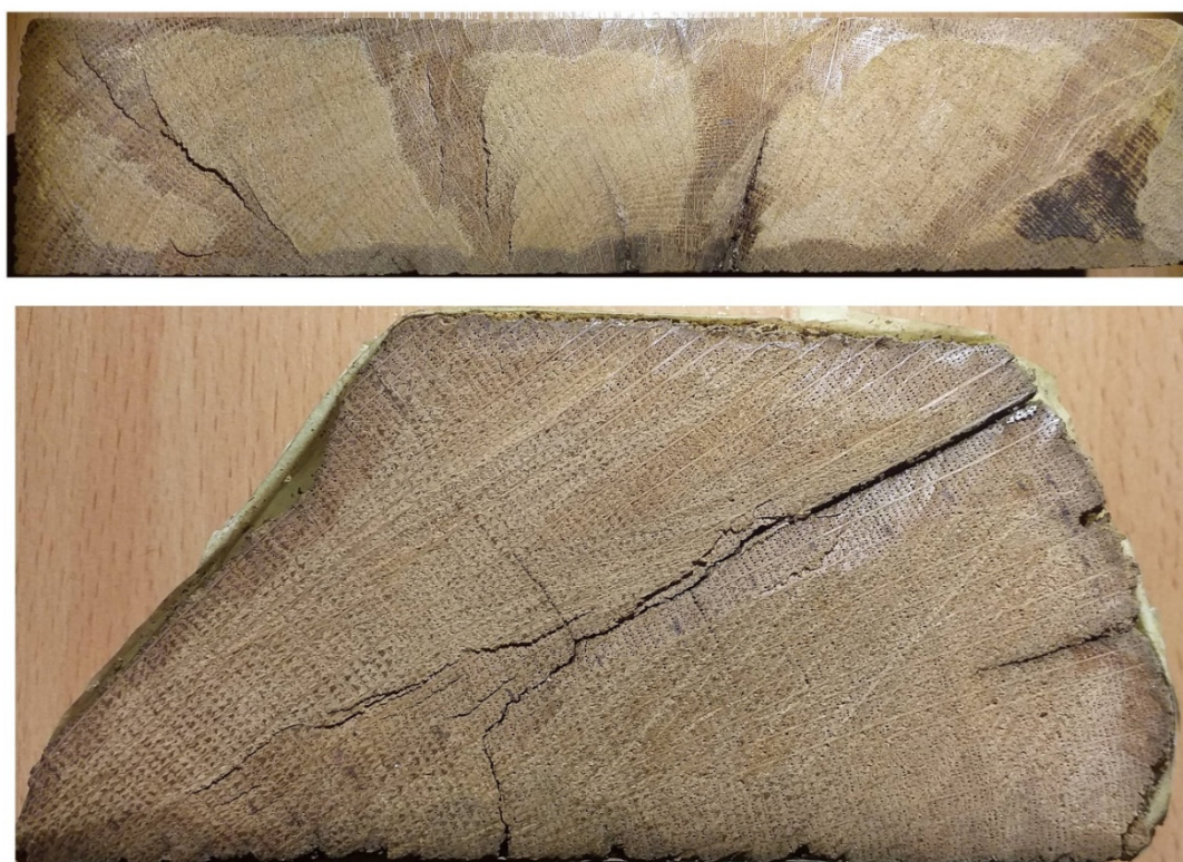
Figure 7. Two of the examined warehouse oak planks with narrow rings but no presence of sapwood rings.
