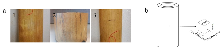
Figure 1. Bamboo specimens: (a) bamboo blocks, (b) bamboo specimen preparation.
