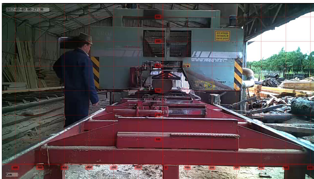
Figure 1. A frame extracted from the Kinovea® software showing the camera's field of view, scalar coordinate system (red) and the tracker placement (yellow).
