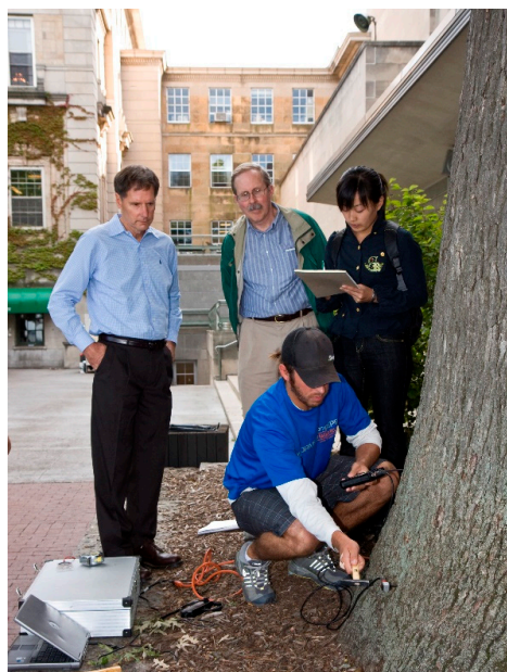
Figure 2. On-site tree inspection with a portable stress wave timer.
