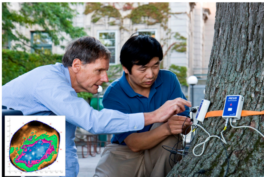
Figure 3. Multi-sensor acoustic tomography test to determine the extent and location of internal defects on a large tree.
