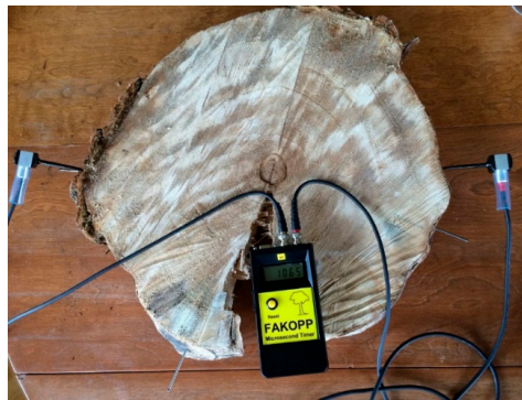
Figure 1. Concept of single-path acoustic method measuring time-of-flight on a tree disk.
