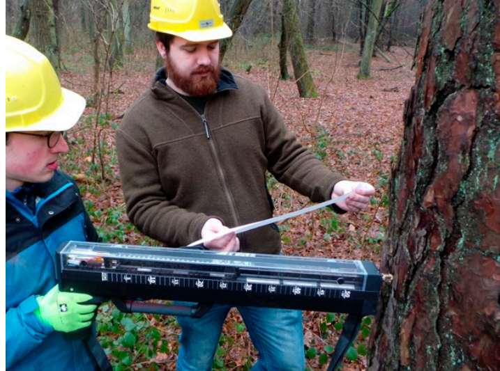
Figure 4. Using a Resistograph® tool to determine the internal condition of a tree (Photo credit: Frank Rinn).
