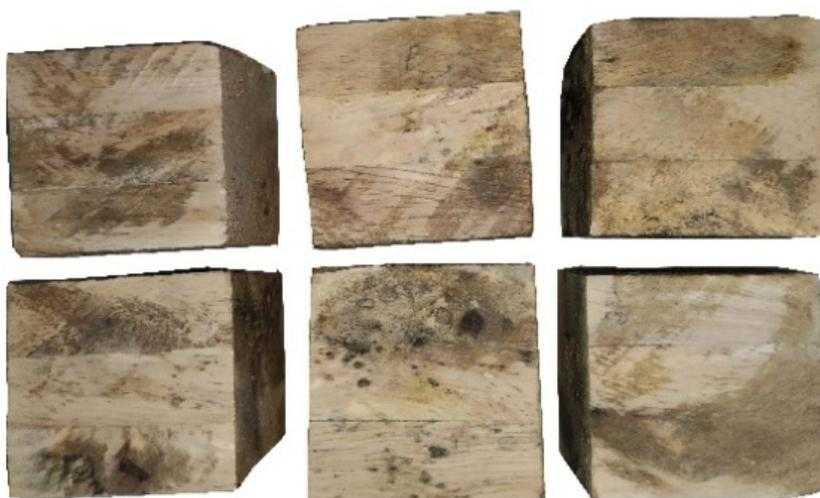
**Figure 6.** Tested delamination specimens in hot water of polystyrene rubber-wood glulam.
