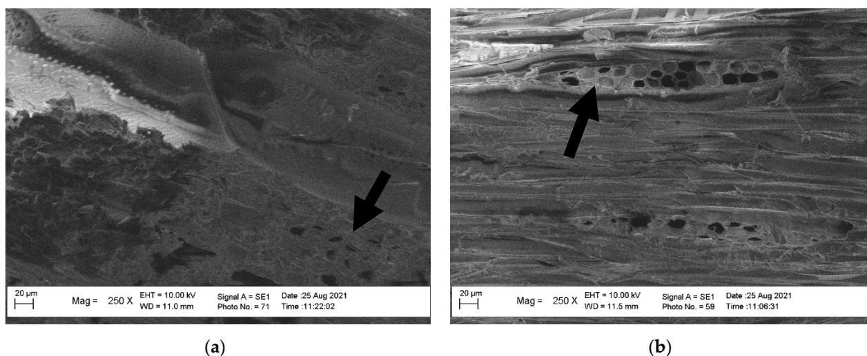
**Figure 4.** Scanning electron microscopy of (a) untreated and (b) polystyrene-impregnated manii wood. Remarks: The arrows indicate the voids.
