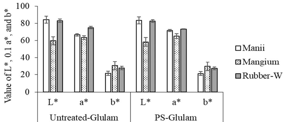
Figure 2. Values of  $L^*$ ,  $a^*$ , and  $b^*$  of the glulam. PS = polystyrene.
