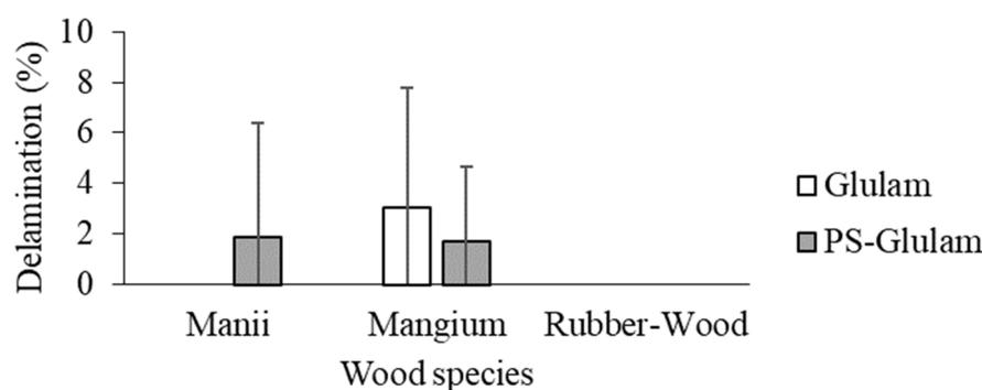
Figure 7. Delamination in hot water of glulam. PS = polystyrene.
