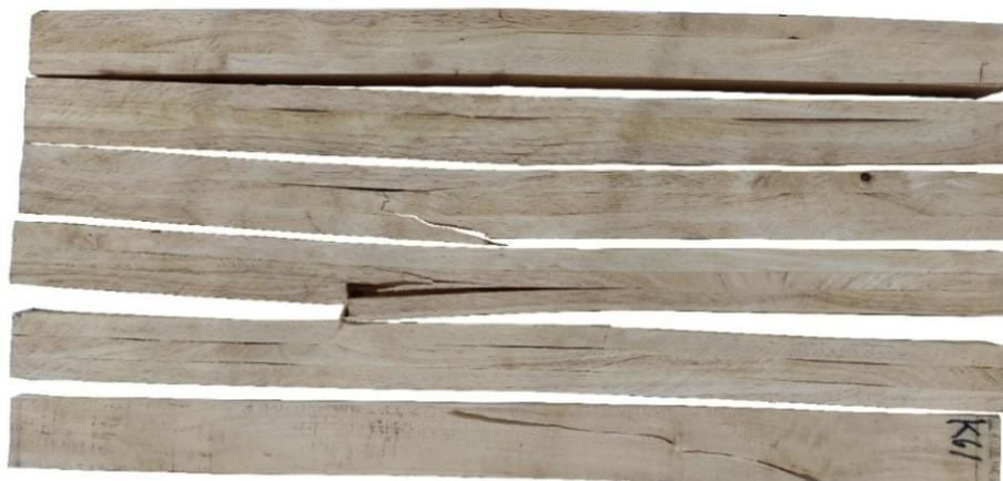
Figure 5. Strength-tested specimens of polystyrene-impregnated rubber-wood glulam.
