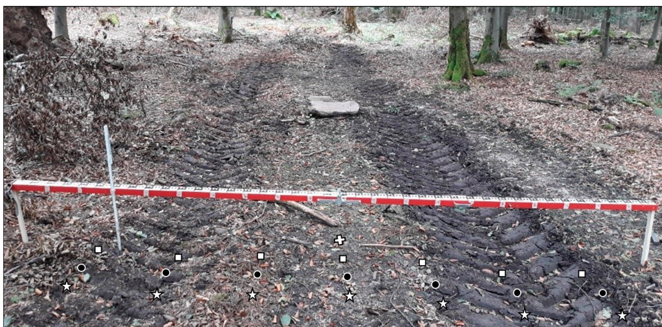
Figure 2. Example of a cross-sectional measuring transect on a machine operating trail. In-situ measurements were performed in advance of the regularly planned CTL thinning operation, using a Penetrologger (squares), vane tester (circles), a dual-mass dynamic cone penetrometer (cross) and a TDR probe (asterisks) as described in Section 2.3.3. The levelled reference beam, positioned on wooden pegs and a yardstick were used to determine rut depth (Figure 3), as it occurred during the given operation.
