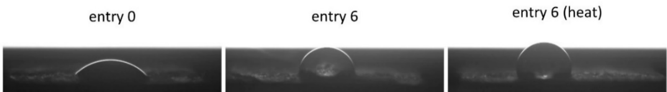
Figure 8. Contact angles for water droplets after 11 s on degreased wood (entry 0), benzylated wood (entry 6), and heat-treated benzylated wood (entry 6 (heat)) surfaces.
