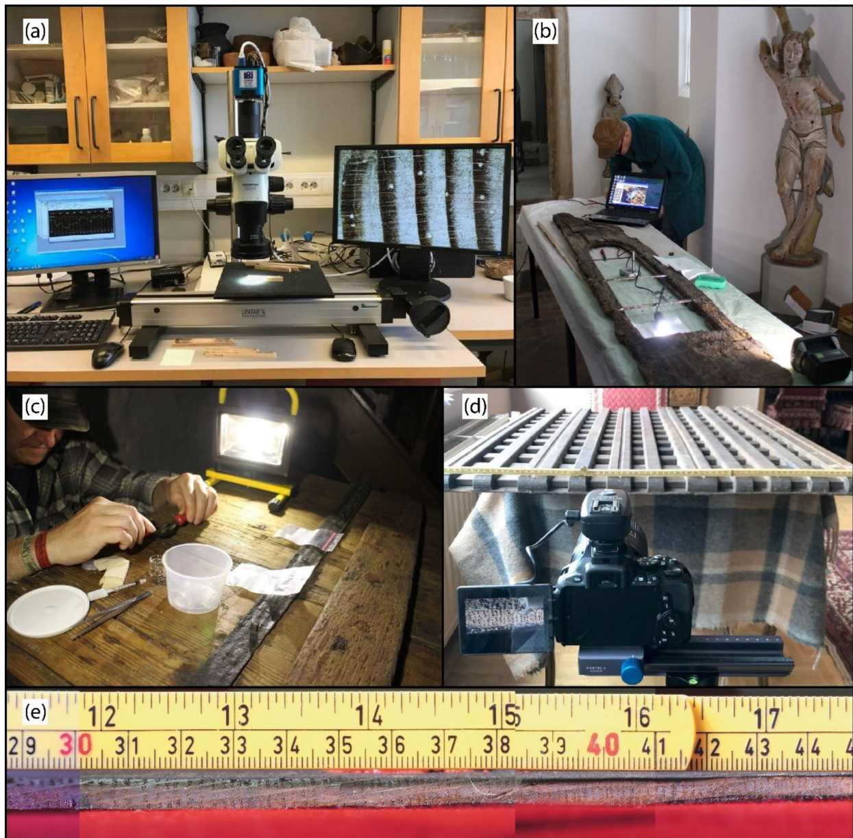
Figure 1. (a) Tree-ring measurements directly on a core from a pine tree. (b) Micro-invasive image analysis on a window frame from Ignaberga church based on high resolution images taken with USB-microscope. (c) Measurement on a horizontal door leaf. In parallel with the measurements small wood samples were taken to allow for radiocarbon dating if the dendrochronological analysis would not yield a reliable result. (d) Micro-invasive image analysis on an oak panel based on high resolution macro photos. Note the magnified annual rings on the camera screen. (e) Composite pictures of an oak plank from macro photos. The scale is helpful when the images are to be linked together and to calibrate the image before the annual rings are to be measured.
