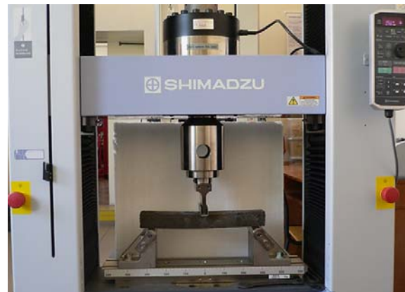
Figure 5. Bending test of the sample.
