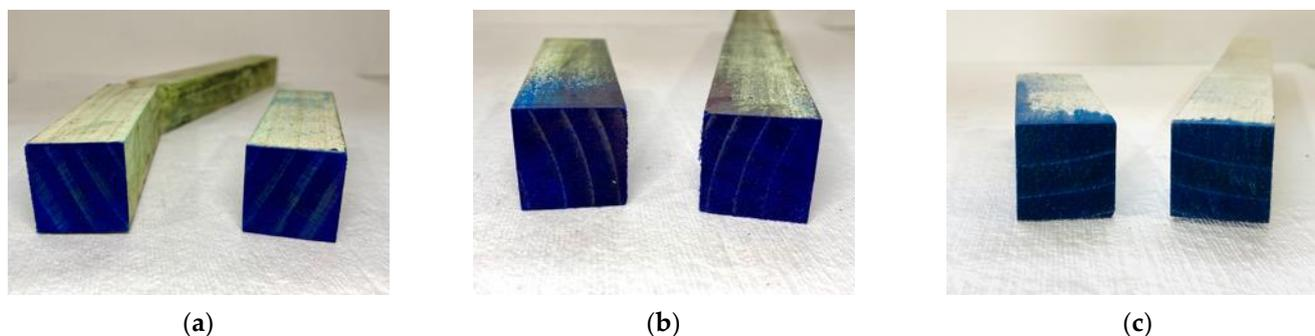
**Figure 2.** Copper penetration in treated wood. Blue color indicates copper in (a) K1 CuNP-treated wood, (b) K2 CuNP-treated wood and (c) micronized-copper-treated wood.
