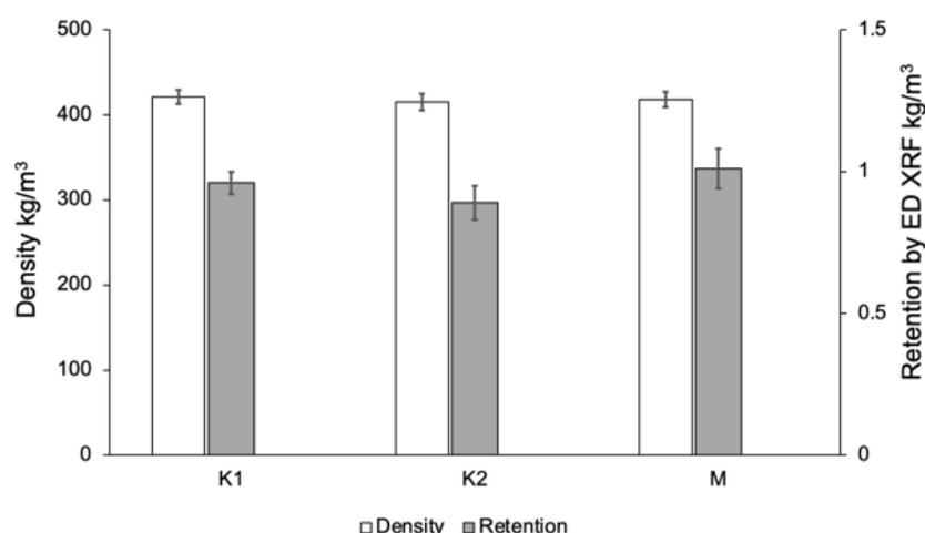
**Figure 1.** Density (primary axis) and Retention by ED XRF (secondary axis) of radiata pine wood impregnated with K1, K2 and M. The maximum standard error for density was 10 kg/m<sup>3</sup> and 0.07 kg/m<sup>3</sup> for ED XRF retention.
