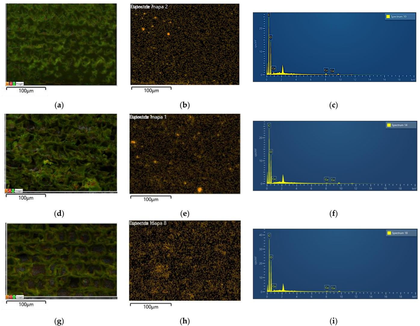
**Figure 3.** SEM-EDS map for copper of (a,b) K1-treated wood, (d,e) K2-treated wood and (g,h) micronized-copper-treated wood. EDS spectrum of K1 (c), K2 (f) and M (i).
