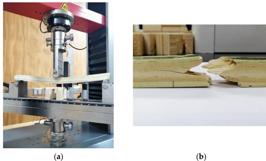
**Figure 4.** Photographs of the static bending test: (a) load applied to an impregnated wood sample by the Zwick/Roell Z020 universal testing machine and (b) failure generated in the specimen after the test was completed.
