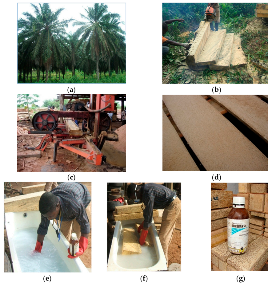
Figure 1. Preparation of study specimens. (a) Oil palm plantation; (b) Converting oil palm logs into beams; (c) Wood-Mizer converting beams into boards; (d) Oil palm lumber; (e) Adding Dursban into water; (f) Immersion of oil palm lumber into preservative; (g) Dursban 4E.
