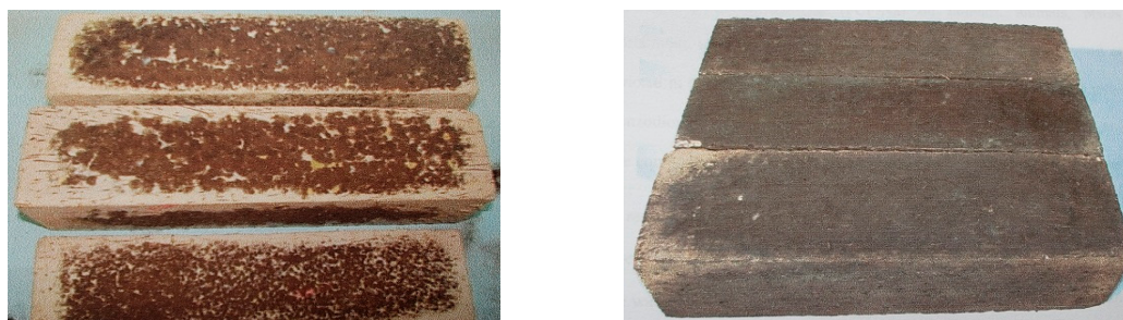
Figure 6. Mildew grows on the surface of the oil palm lumber and discolors the affected specimen to black.
