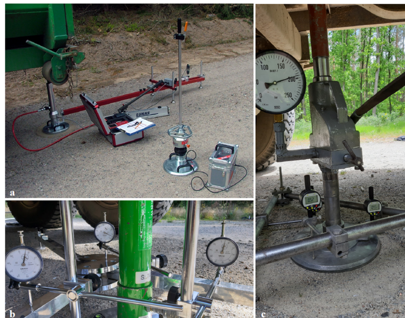
Figure 2. Equipment used for measuring the bearing capacity of forest roads: (a) light falling weight deflectometer Zorn ZFG 3000 GPS (foreground), and static load plate HMP PDG Pro (background); (b) static load plate VSS-3P-000 with 3 analogue displacement sensors; (c) static load plate VSS-3P with 3 electronic displacement sensors (Photos: S.M. Grajewski).
