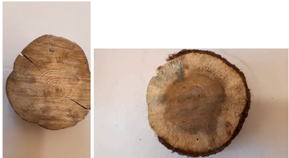
Figure A2. Cross-section of pine and oak wood samples taken from rollers from research sections in 2022.
