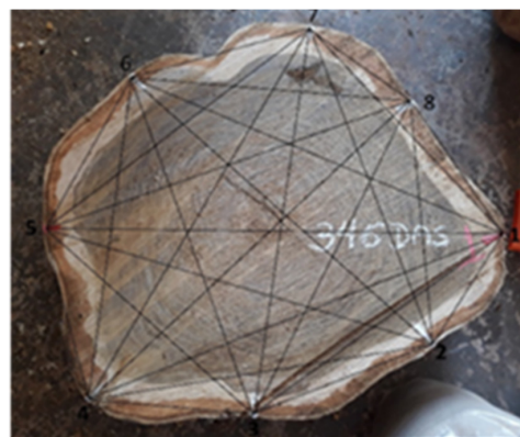
Figure 6. Example of theoretical routes of the projected measurement mesh on the face of the disc.
