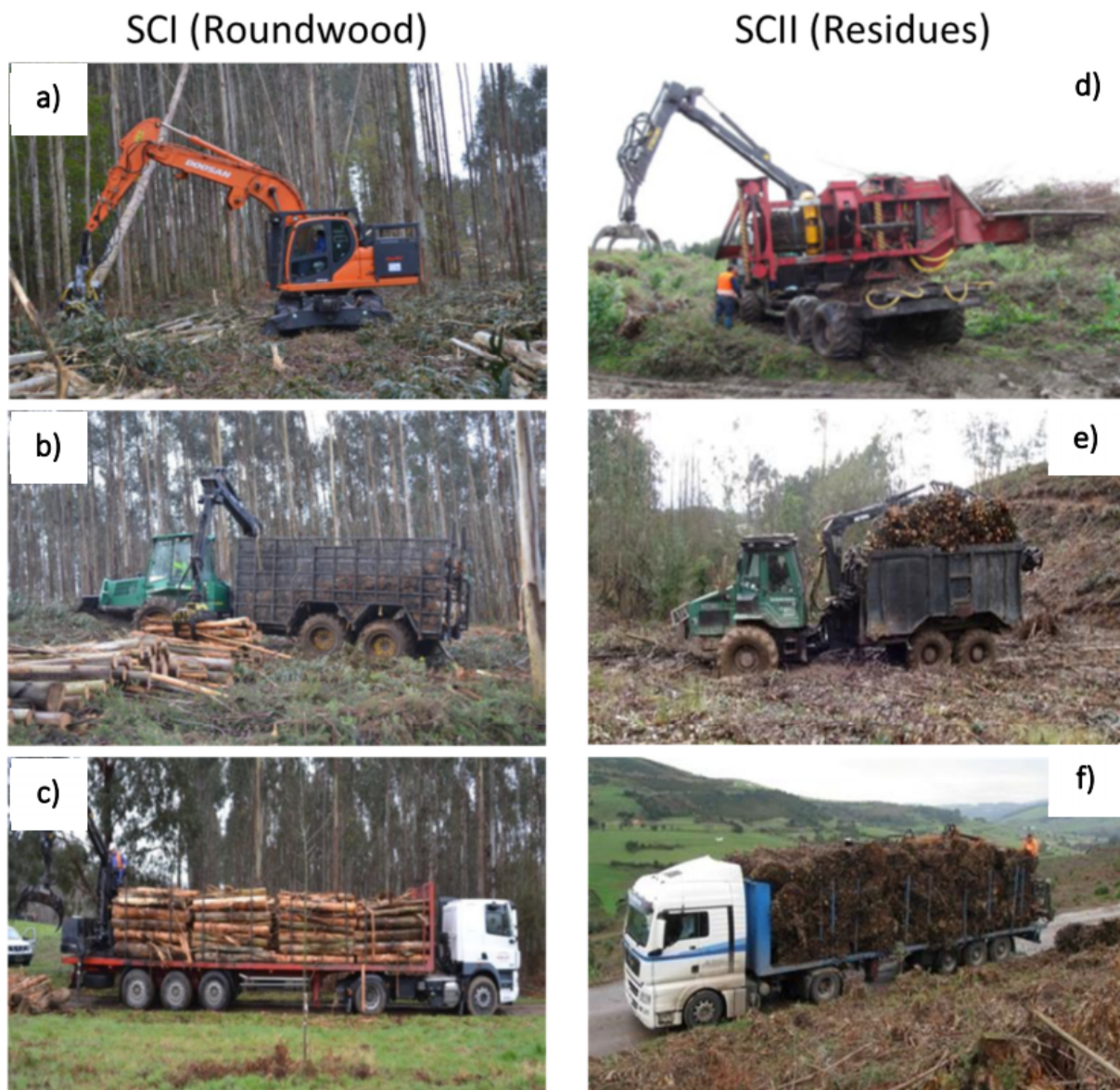
Figure 3. Equipment used in SCI and SCII: (a) Tree felling, debarking, debranching, (b) extraction of logs, (c) transport of logs, (d) bundling, (e) extraction of bundles, (f) transport of bundles.
