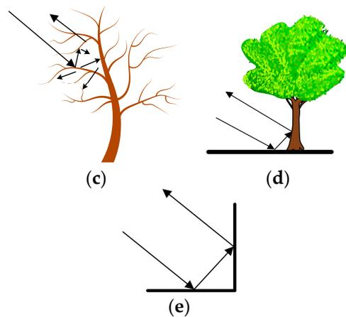
**Figure 3.** Basic physical radar backscattering mechanisms: (a,b) single surface backscattering, (c) volume, and (d,e) double dihedral.
