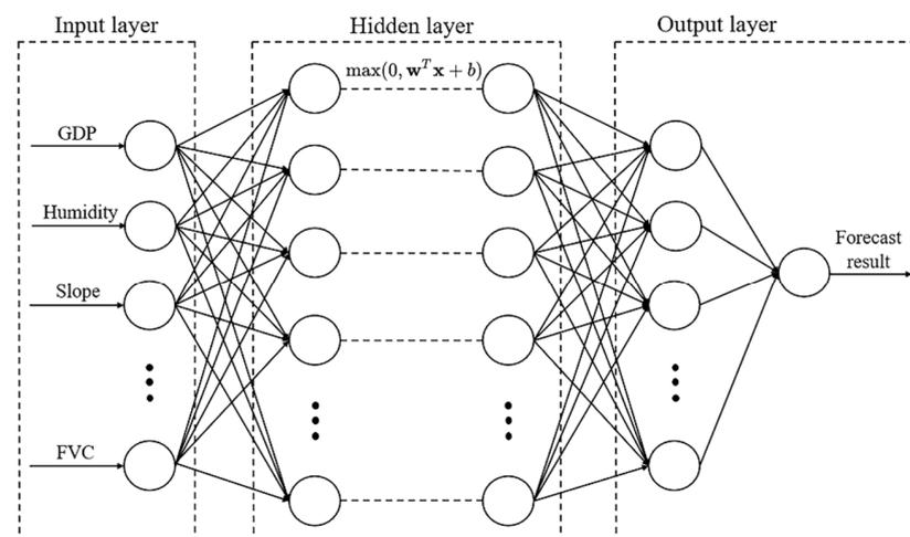
**Figure 4.** Schematic diagram of the artificial neural network for predicting the probability of forest fire.
