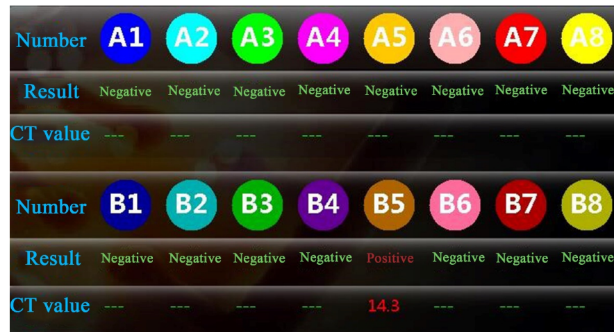
Figure 5. The results of detection of different nematodes by EMA. A1–A8 and B1–B6 are the well numbers, and the corresponding test samples of wells A1–A8 are Bm01–Bm08. The corresponding test samples of wells B1–B4 are Bm09, Bm10, Bs01 and Bv01, respectively; well B5 is the positive control, and well B6 is the negative control. B7 and B8 are empty slots.
