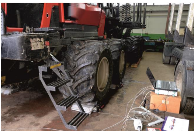
Figure 3. Determining the centre of gravity of the forwarder in (A) horizontal plane and (B) on slope.
