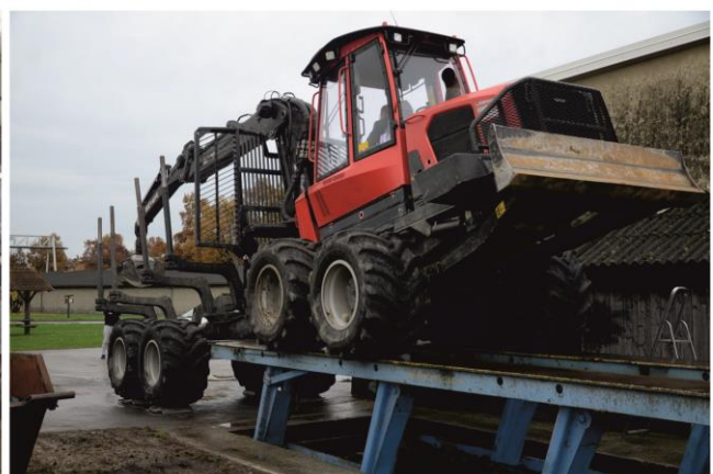
Figure 3. Determining the centre of gravity of the forwarder in (A) horizontal plane and (B) on slope.
