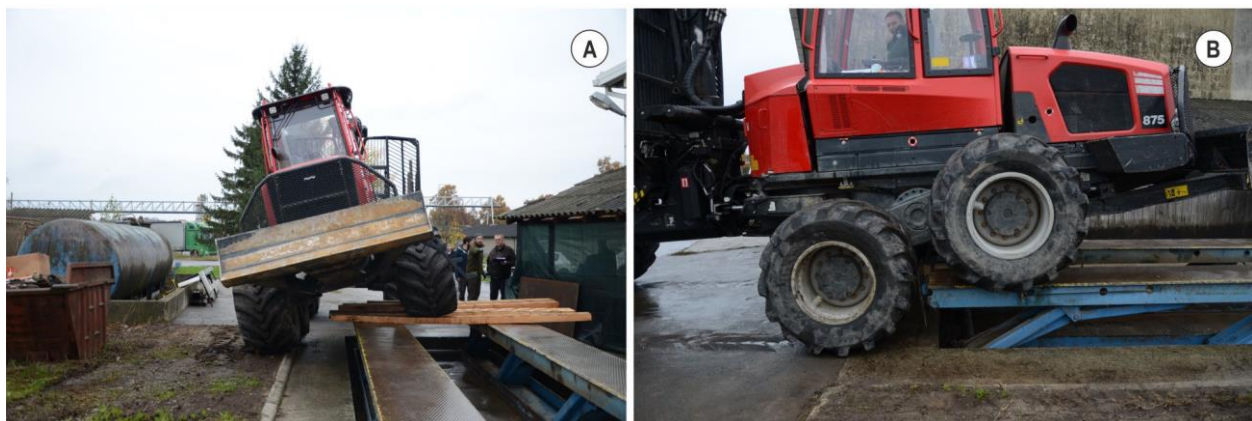
Figure 8. Measurement of frame oscillation (A) and bogie axle assembly wheelbase angle (B).
