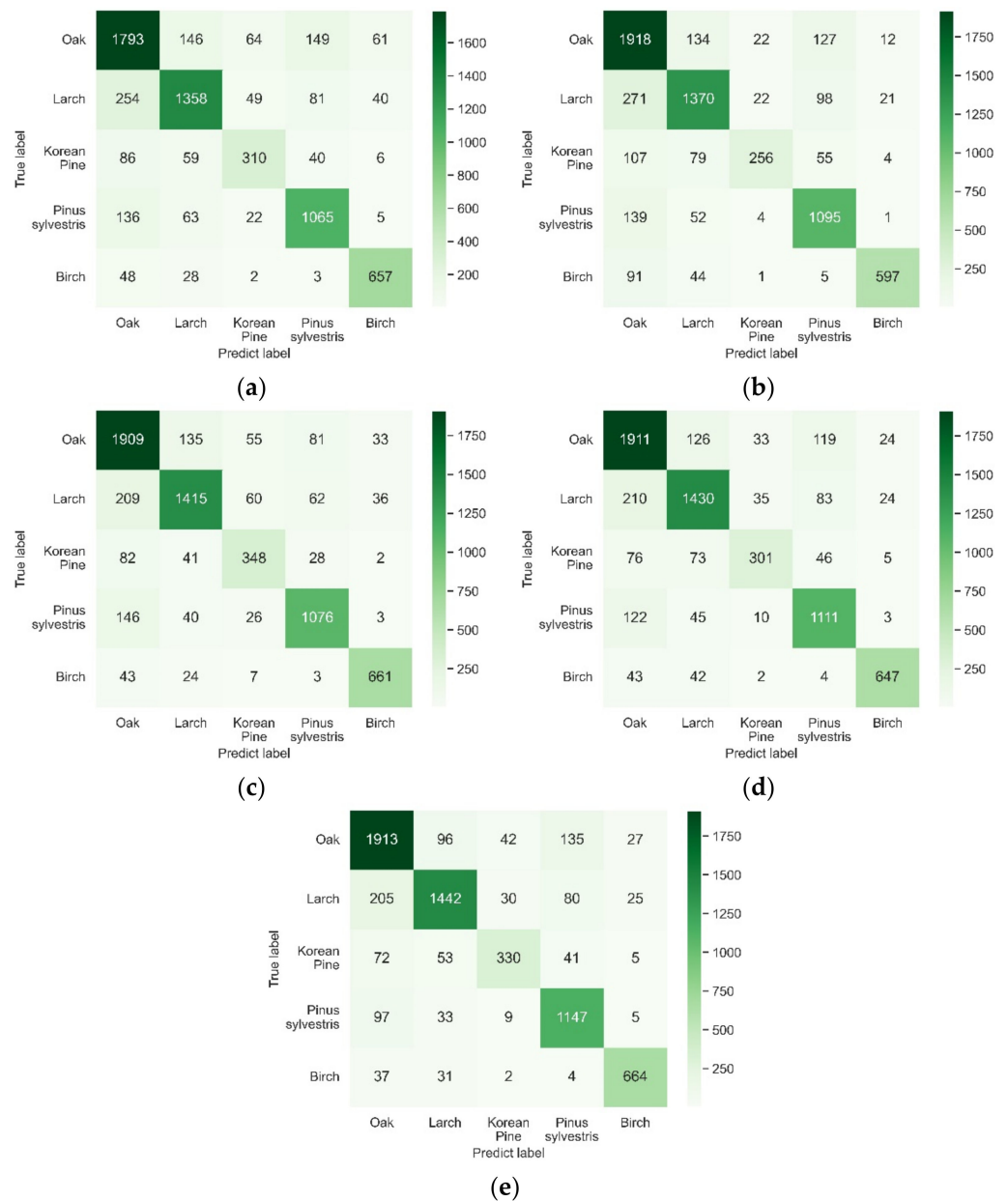
Figure 10. Confusion matrix for various classification methods: (a) KNN; (b) RF; (c) ANN; (d) LightGBM; (e) ensemble.
