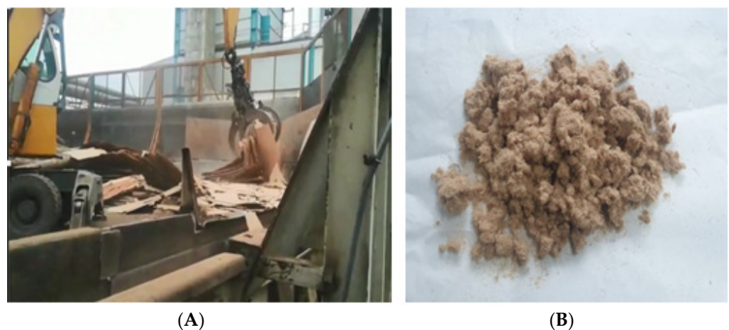
Figure 1. (A) The scraps of the waste MDF. (B) Recycled fibers obtained from the waste MDF.
