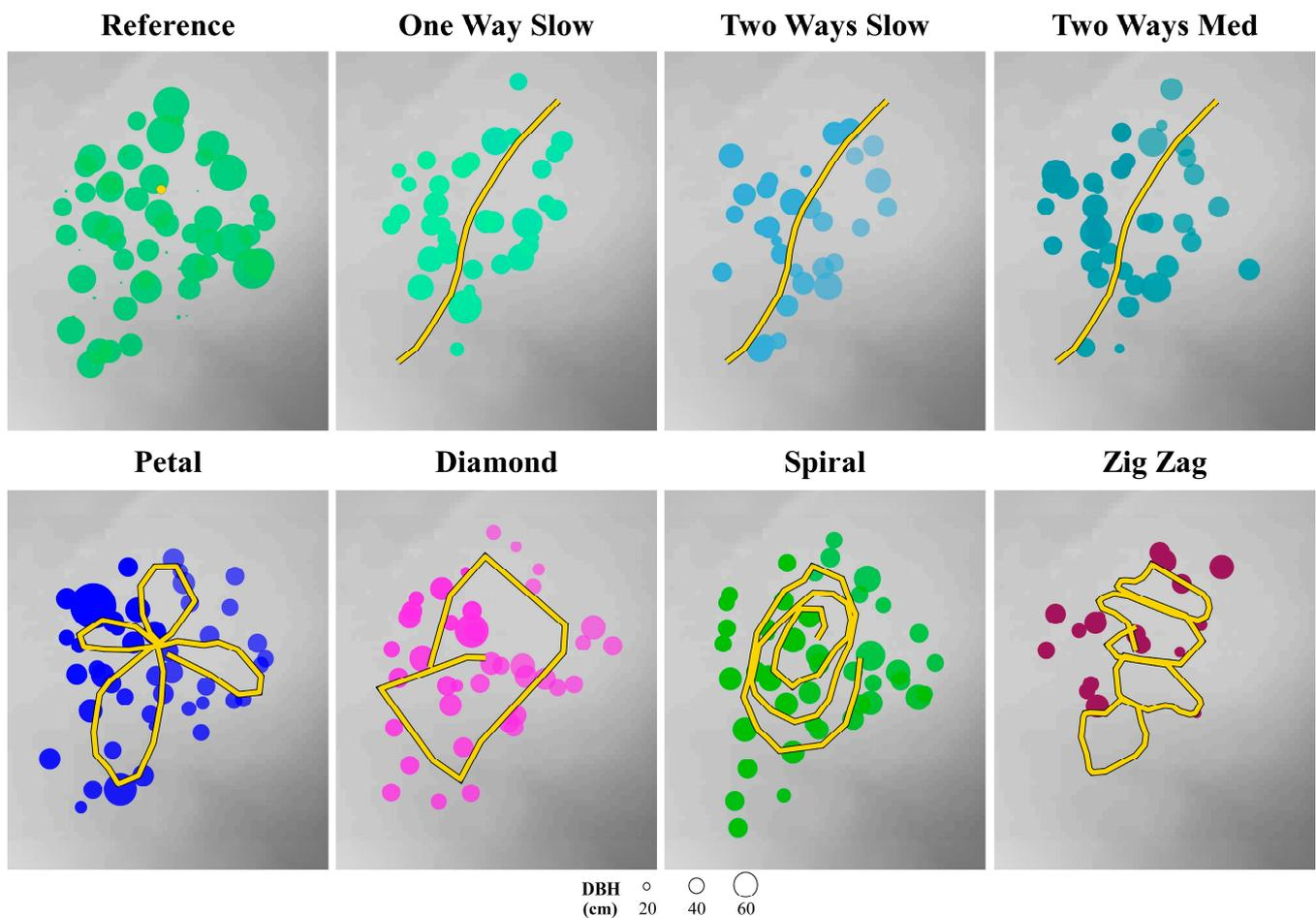
**Figure 4.** Maps of single tree acquired by total station (Reference) and by the different SPOT protocols. The real walking path did not coincide with the theoretical path (Figure 3) due to the presence of obstacles on the ground (such as stems, regeneration trees, dead wood, etc.), which are typical in seminatural environments [27].
