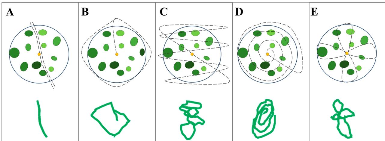
**Figure 3.** Field acquisition paths: (A) transect; (B) diamond; (C) zig-zag; (D) spiral; (E) petals. Above is the planned protocol in a hypothetical scenario, a distribution of simulated trees is shown in green, and below the SPOT recorded path.
