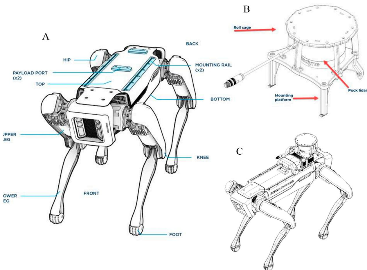
**Figure 2.** (A) major parts of SPOT; (B) Spot Velodyne LiDAR; (C) mounting the payload on the SPOT platform (adapted from <https://support.bostondynamics.com/s/article/Spot-anatomy> accessed on 14 July 2023).
