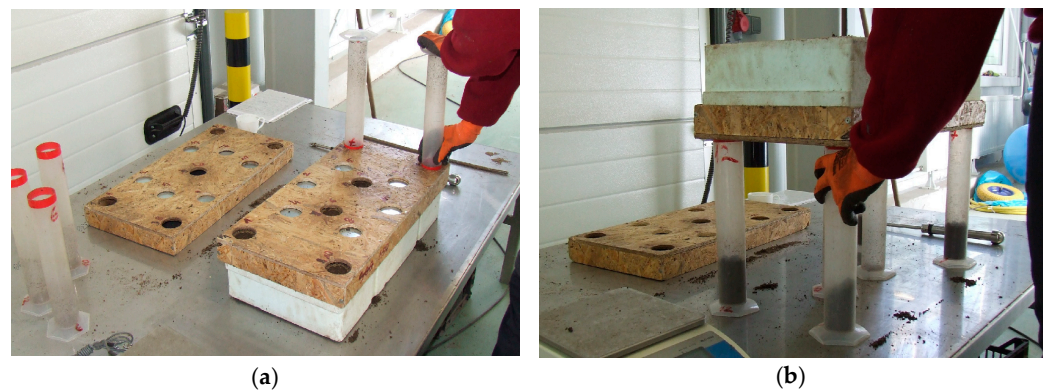
Figure 4. Measurement of bulk density in container cells. A collector with volumetric cylinders mounted on a container (a), pouring the substrate into the cylinders (b). Photo: M. Kormanek.
