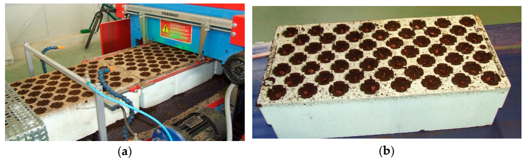
Figure 2. Filling the V150 container with substrate (a) and the V300 container filled with substrate and sown (b). Photo: M. Kormanek.
