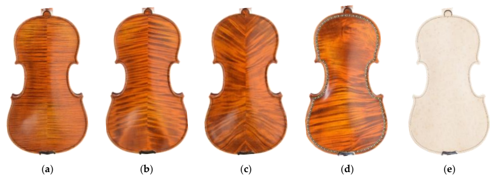
Figure 1. The common figures of sycamore maple wood: (a) curly grain; (b) fiddleback figure; (c) flame grain; (d) partial quilted grain; (e) bird’s eye figure.
