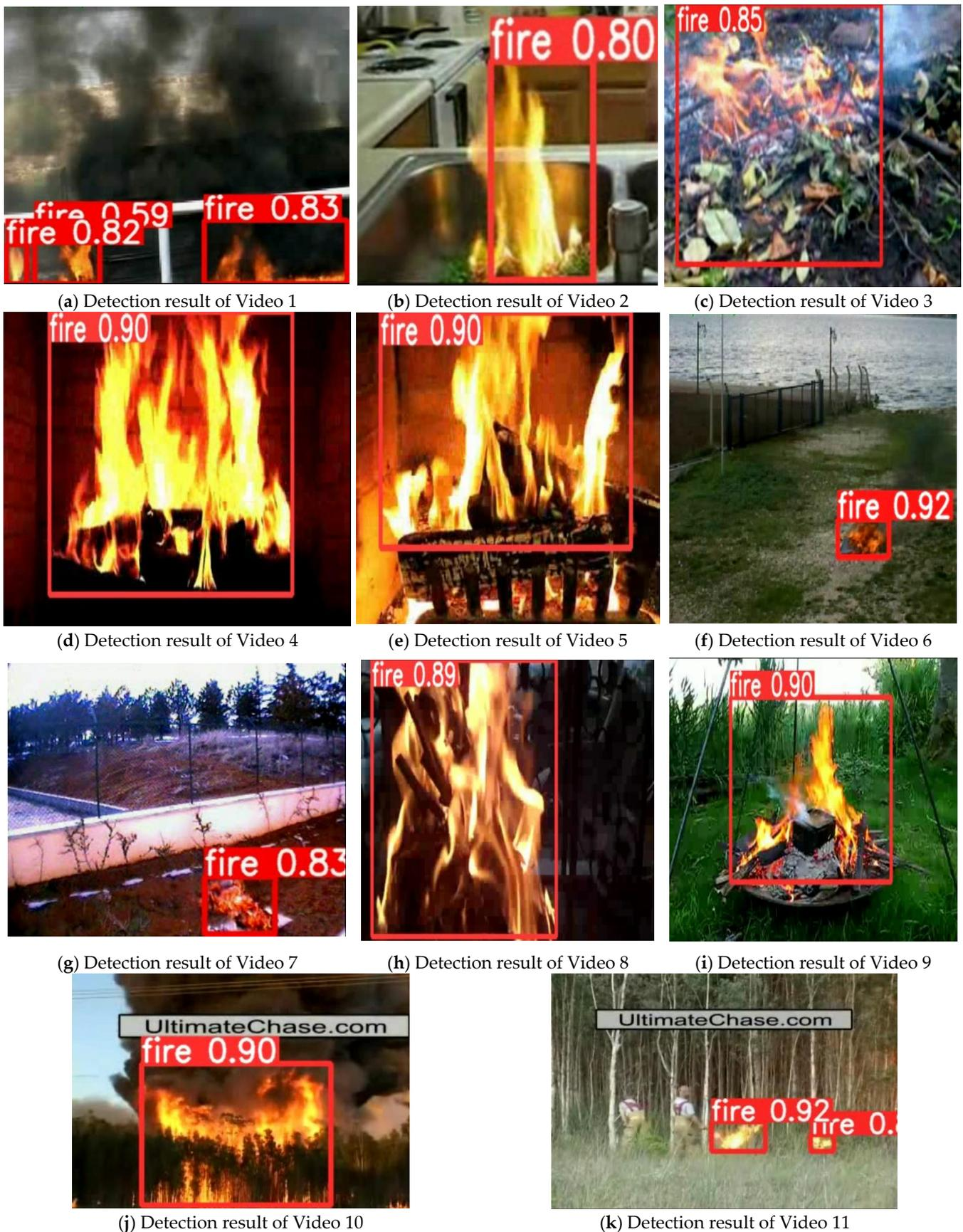
**Figure 15.** Slicing of the public fire video dataset VisiFire detection results. (a–k) are slices of the results of detecting the 1st to 11th fire videos in VisiFire, respectively.
