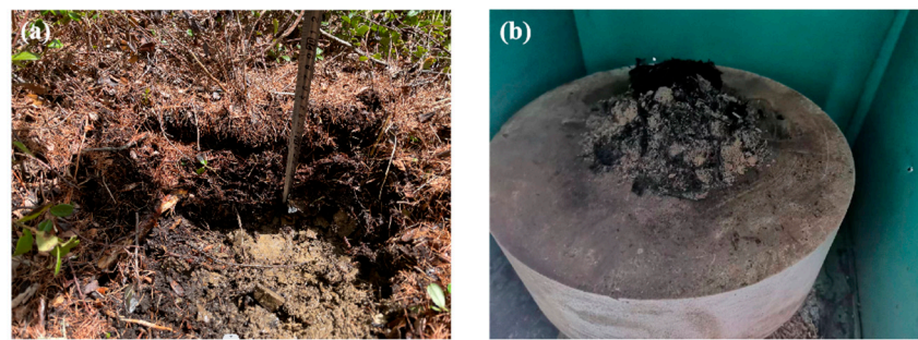
Figure 2. Soil sample before and after the smouldering combustion experiment: (a) before combustion; (b) after combustion.
