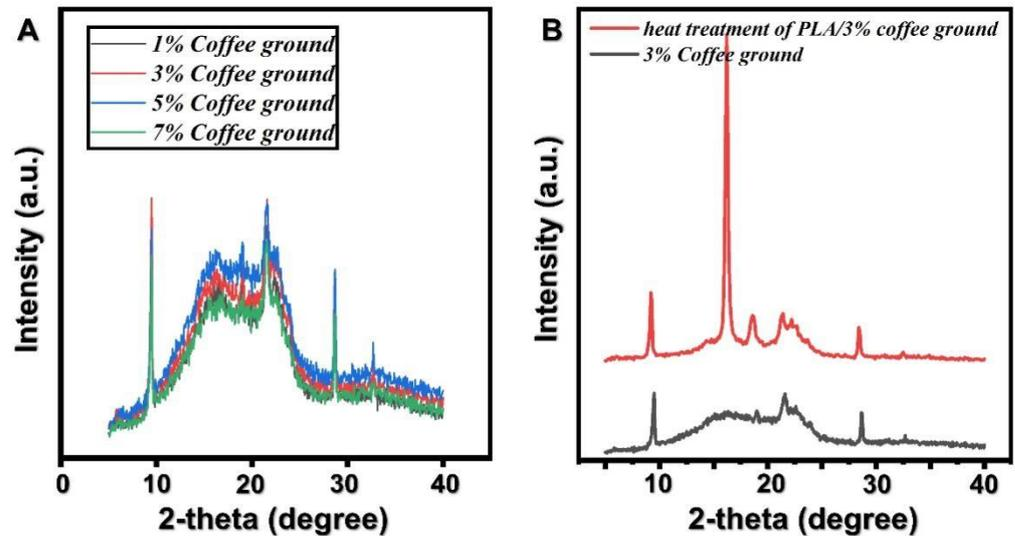
**Figure 6.** XRD curves of different PLA/coffee grounds 3D printing materials: (A) XRD curves of 1%, 3%, 5%, and 7% coffee grounds 3D printing products; (B) XRD curves of 3% coffee grounds 3D printing products and thermal treatment of PLA/3% coffee grounds 3D printing products.
