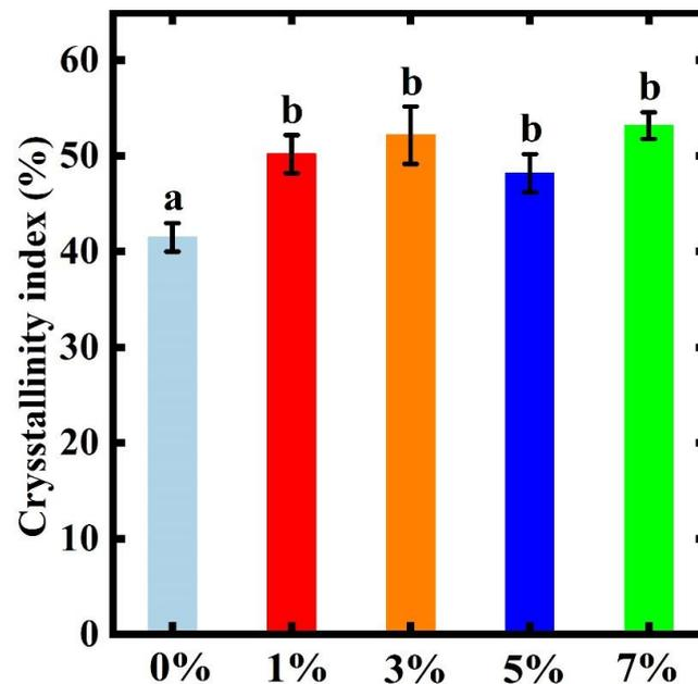
**Figure 7.** The crystallinity index of different PLA/coffee grounds 3D printing materials. Lowercase letters indicate significant differences between groups ( $p < 0.05$ ). The error bar represents the standard deviation.
