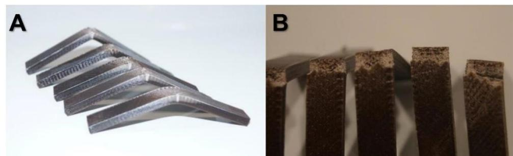
**Figure 4.** The standard bending specimen of PLA/coffee grounds after the bending test: (A) PLA/3% coffee grounds composite 3D printing products; (B) PLA/7% coffee grounds composite 3D printing products.
