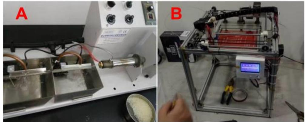
**Figure 1.** (A) Drawing machine; (B) FDM 3D printer.
