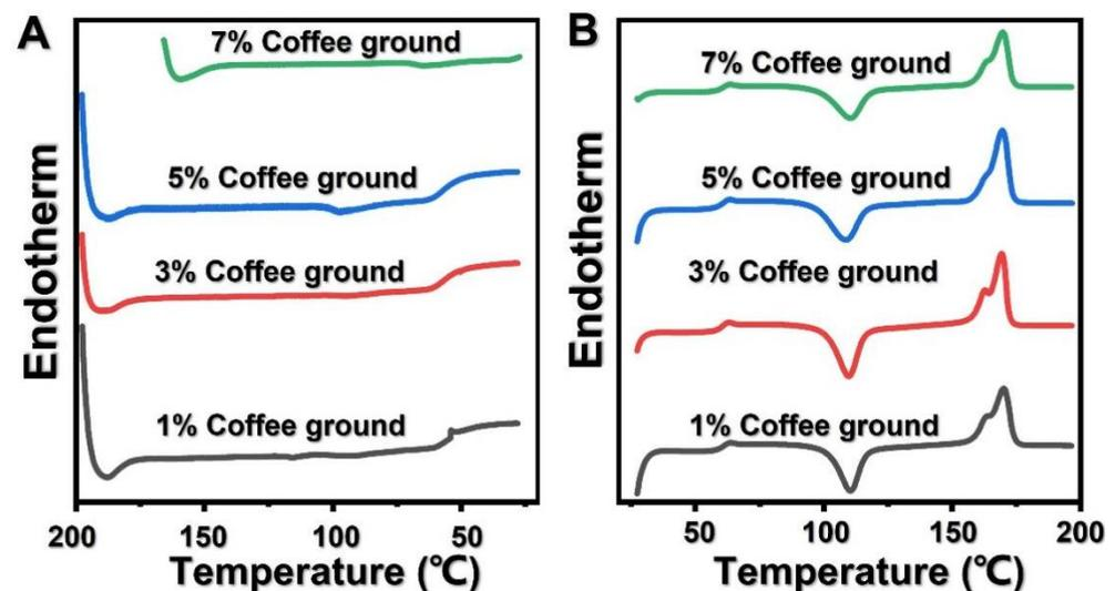
**Figure 8.** The DSC curves of different PLA/coffee grounds 3D printing products: (A) the cooling process of PLA/coffee grounds 3D printing products with different coffee grounds additions; (B) the second heating process of PLA/coffee grounds 3D printing products with different coffee grounds additions.
