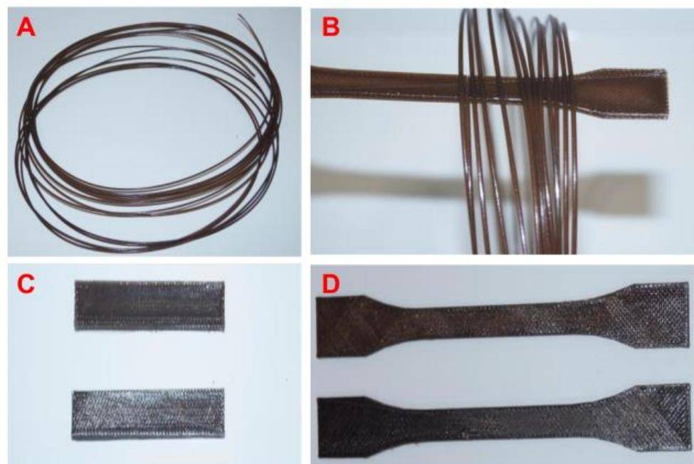
**Figure 2.** (A,B) Three-dimensional printing wire produced with coffee grounds; (C,D) standard specimens for the mechanical properties test.
