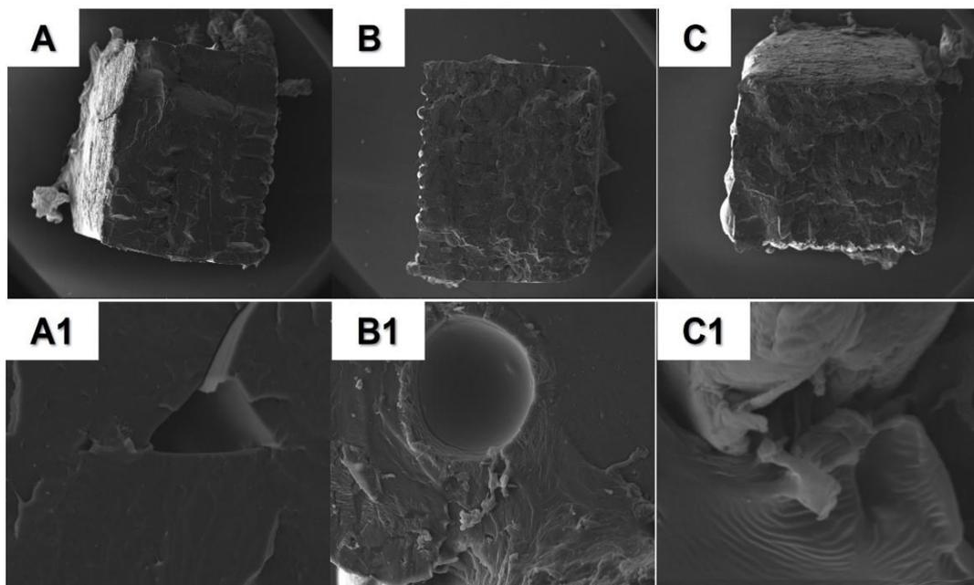
**Figure 5.** SEM images of PLA/coffee grounds composite 3D printing products with different coffee grounds additions: (A,A1) PLA composite 3D printing products; (B,B1) PLA/3% coffee grounds composite 3D printing products; (C,C1) PLA/7% coffee grounds composite 3D printing products.
