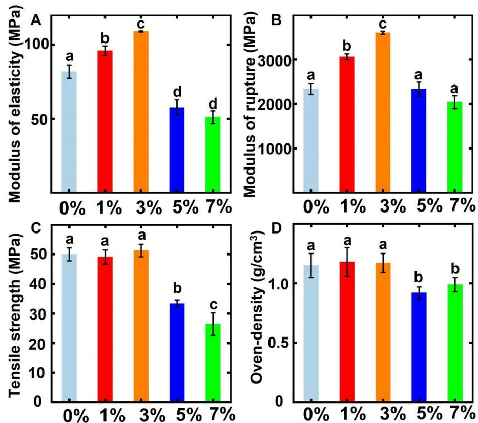
**Figure 3.** Physical/mechanical properties of PLA/coffee grounds composite 3D printing products: (A) modulus of elasticity; (B) modulus of rupture; (C) tensile strength; (D) oven density. The figure shows significant differences between groups ( $p < 0.05$ ). The error bar in the figure represents the standard deviation.
