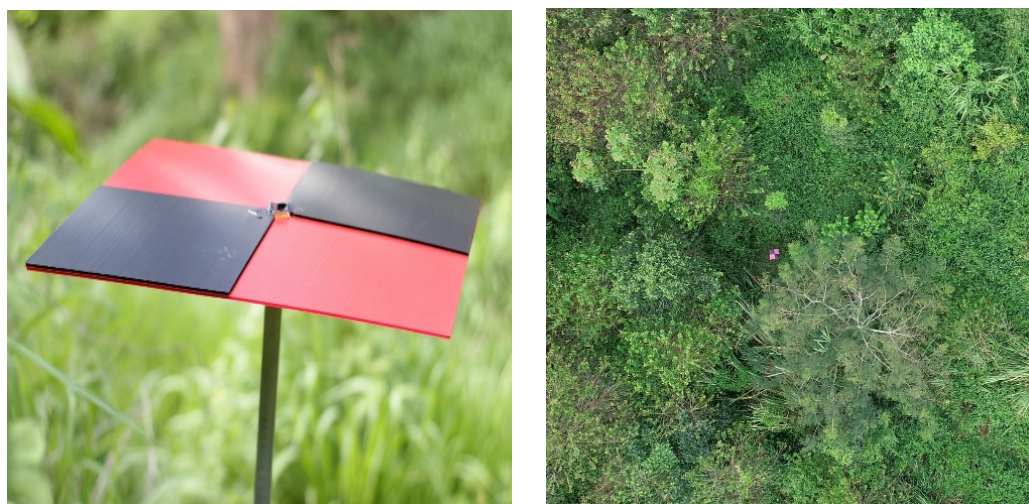
Figure S1. (Left) red-black ground-marker placed in the center of circular sample plots, (Right) red-black ground marker, detected by drone image sensing.
