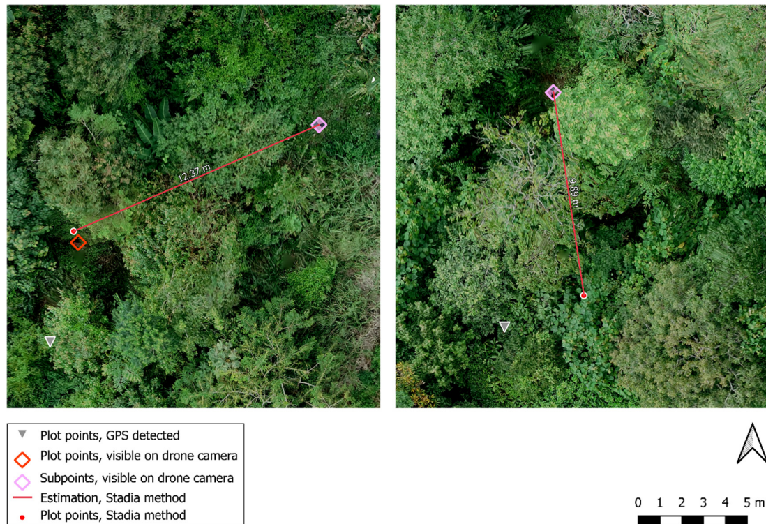
Figure S5. Examples of stadia method and comparisons with GPS-detected points in orthophoto. (Left) Plot point was visible on drone-derived image (actual plot point; red square) and estimated using stadia method (red point) from visible subpoint (pink square). Two points were closer than the distance between GPS detection (grey triangle) and actual plot point. (Right) ground marker was not visible, and plot point was estimated using stadia method. Stadia method was applied in three sites, where it was necessary.
