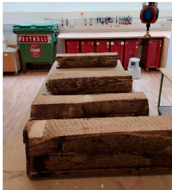
Figure 2. Four Paulownia logs extracted from two trees at different heights (0–1 m, 4.5–6 m).
