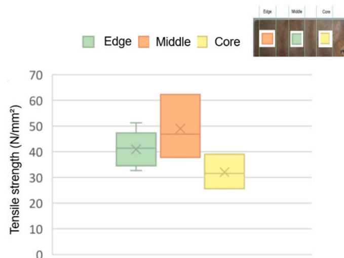
Figure 19. Tensile strength of Paulownia samples extracted from the cross-section.
