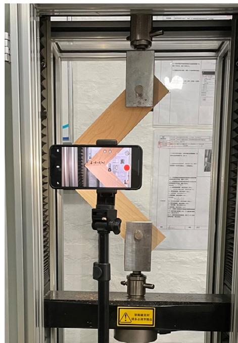
**Figure 4.** Setup for measuring the diagonal tensile strength of the oblique corner joint.
