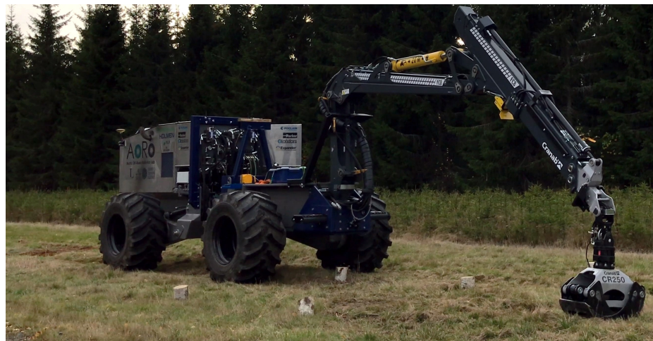
Figure 8. The research platform in the role of the AutoPlant machine during the state timing field experiments. Photograph courtesy of Stina Johannesson.
