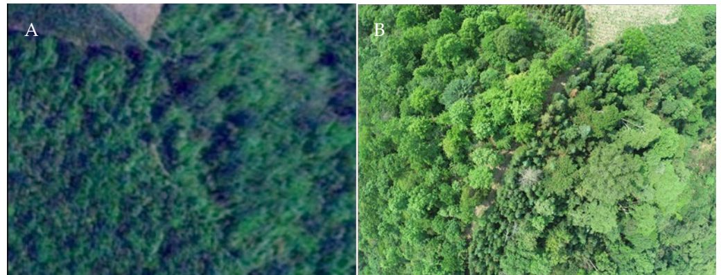
Figure 8. The comparison of satellite remote sensing and centimeter-level UAV-RGB imagery: (A) is a satellite remote sensing image with a spatial resolution of 0.6 m; (B) is the UAV-RGB imagery with a resolution of 3.5 cm.
