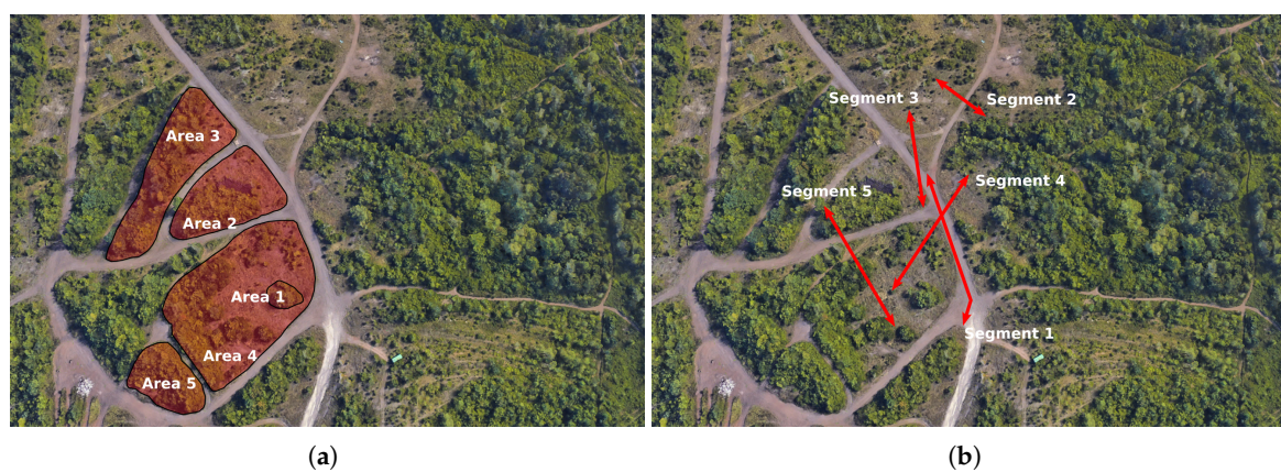
Figure 6. Landmarks and regions used to validate the spatial correctness of the SLAM map. Given the photogrammetry baseline and the SLAM map span different areas, we chose regions that appear in both. (a) shows the specific areas we used to validate the SLAM map which intersect between baseline and SLAM, (b) shows the specific segments or landmarks for detailed comparison
