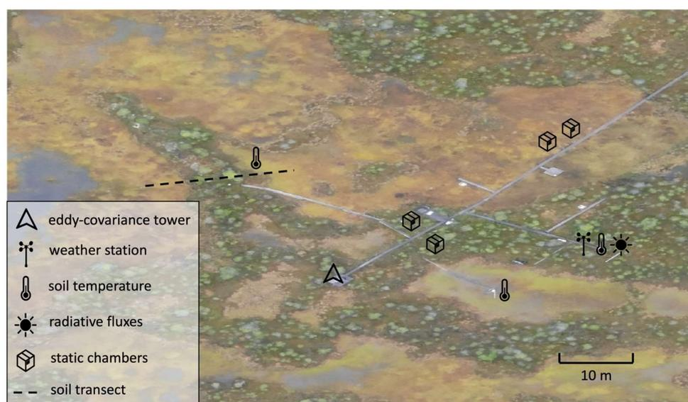
**Figure 2.** The orthophoto of the ridge-hollow site with a detailed view of the instrument placement.
