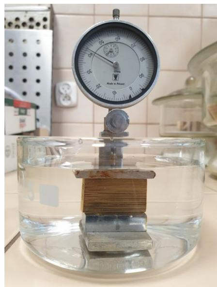
**Figure 2.** A picture of equipment used for the measurement of swelling kinetics.
