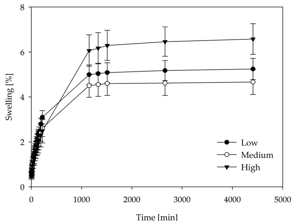
**Figure 4.** Kinetics of linear swelling in the tangential direction measured for three different density groups of bamboo blocks: low, medium, and high; error bars represent the standard deviation.
