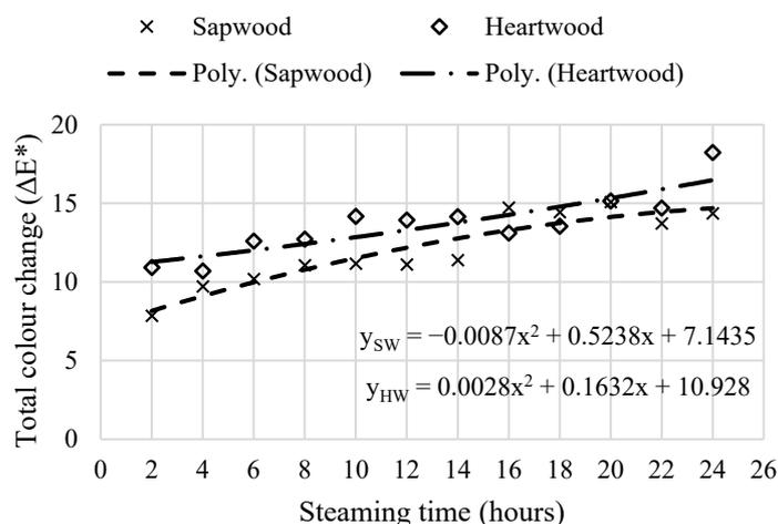
Figure 7. Heartwood and sapwood total color change ( $\Delta E^*$ ) during the steaming process.
