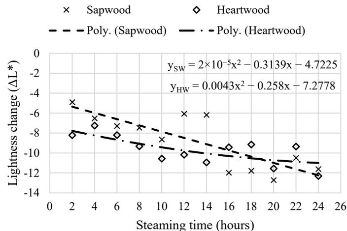
**Figure 4.** Heartwood and sapwood lightness ( $\Delta L^*$ ) change during the steaming process.
