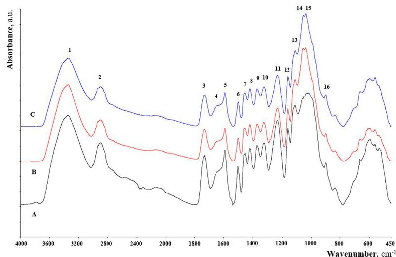
**Figure 10.** FT-IR spectra of un-steamed (A) and heartwood samples steamed for 12 (B) and 24 (C) hours. (Numbers 1 to 16 denote characteristic carbohydrates and lignin bands).
