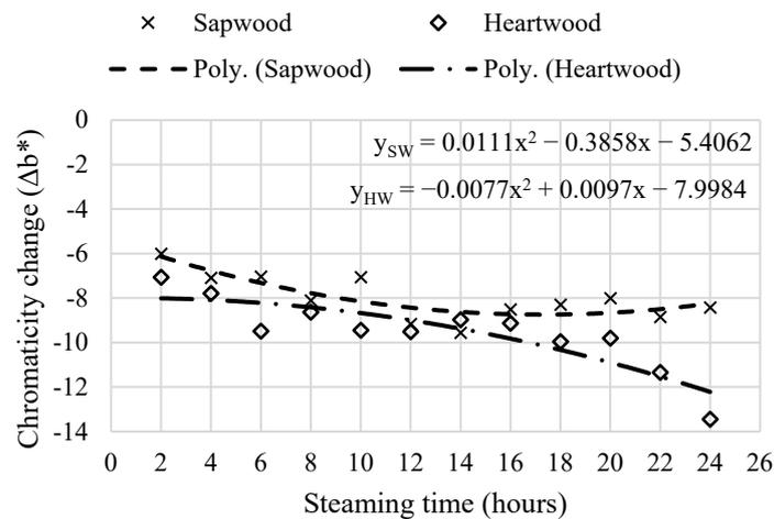
**Figure 6.** Heartwood and sapwood chromaticity components ( $\Delta b^*$ ) change during the steaming process.
