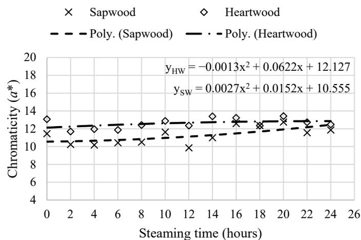
Figure 2. Heartwood and sapwood chromaticity component ( $a^*$ ) trend during the steaming process.
