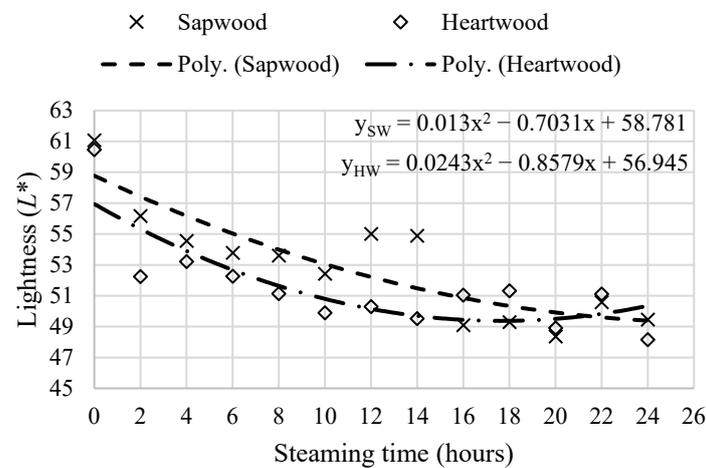
Figure 1. Heartwood and sapwood lightness ( $L^*$ ) trend during the steaming process.
