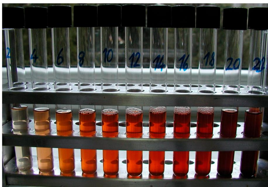
**Figure 8.** Cumulative condensate from the steaming chamber, extraction every two hours (left to right).
