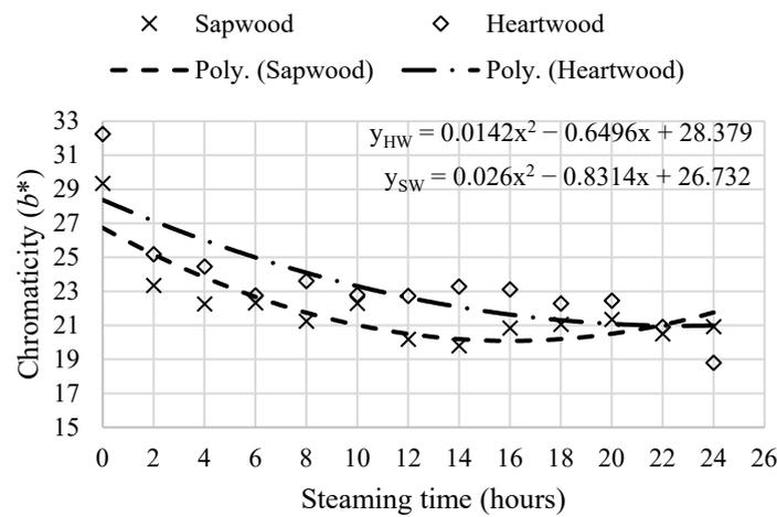
**Figure 3.** Heartwood and sapwood chromaticity component ( $b^*$ ) trend during the steaming process.
