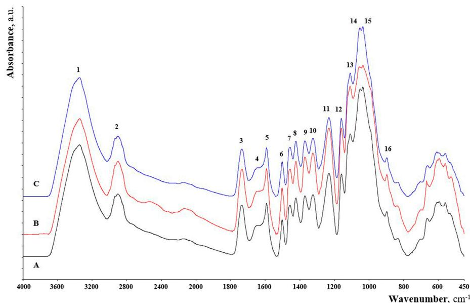
**Figure 9.** FT-IR spectra of un-steamed (A) and sapwood samples steamed for 12 (B) and 24 (C) hours. (Numbers 1 to 16 denote characteristic carbohydrates and lignin bands).
