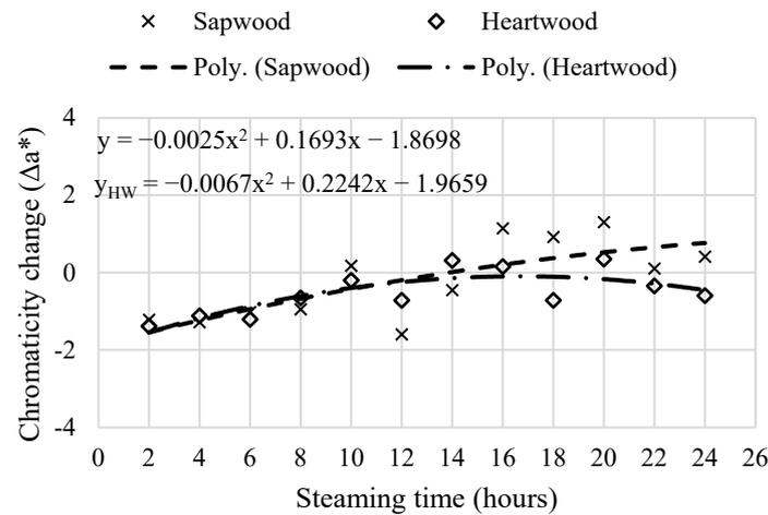
**Figure 5.** Heartwood and sapwood chromaticity components ( $\Delta a^*$ ) change during the steaming process.
