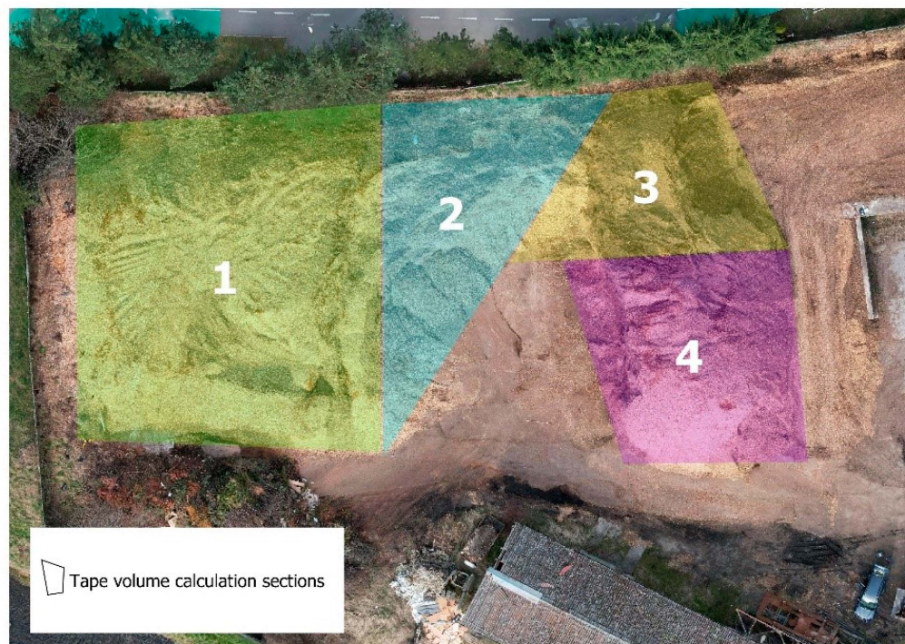
Figure 10. Dividing the pile into sections.
