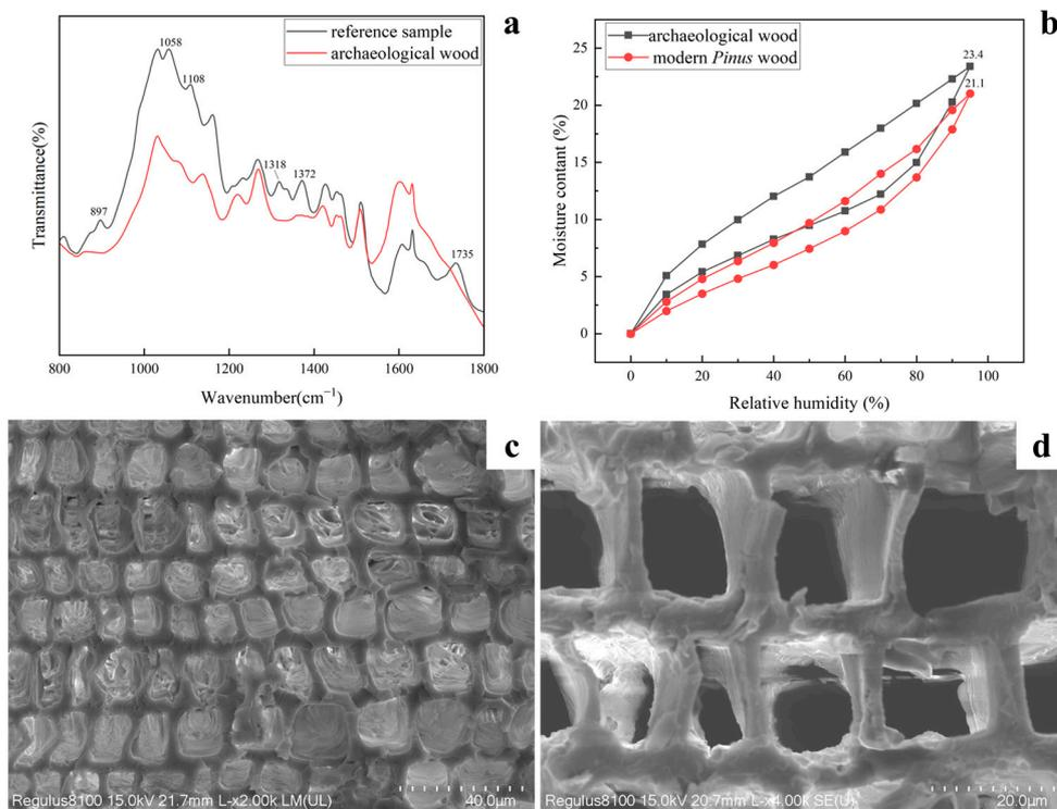
**Figure 3.** FT-IR spectra (a) and DVS curves (b) of the reference sample and archaeological wood; SEM of the archaeological wood ((c): 2000 $\times$ , (d): 4000 $\times$ ).
