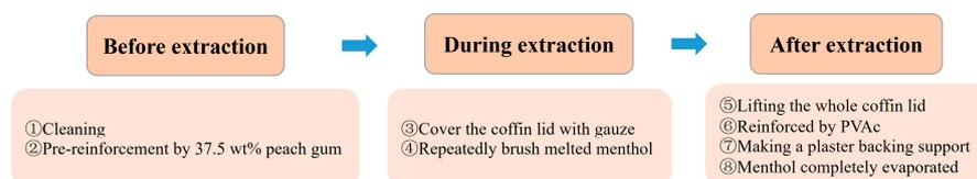
**Figure 7.** The procedure of using menthol as a temporary consolidant in coffin lid extraction.
