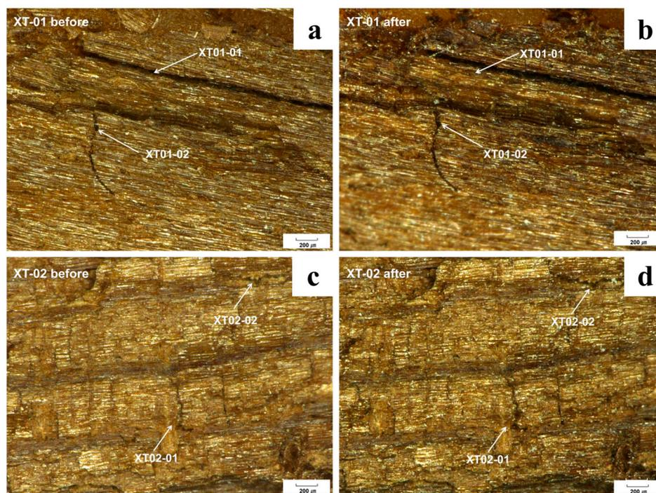
**Figure 5.** Micrographs of samples XT01 and XT02 showing the surface and fissures morphology before (a,c) and after (b,d) menthol treatment (50 $\times$ ).
