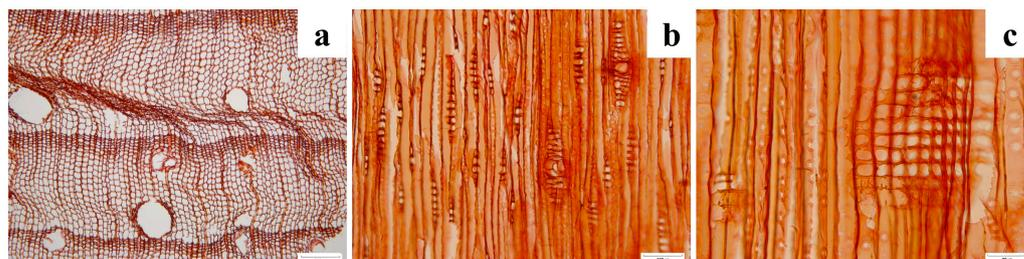
**Figure 2.** Anatomical structure of wood sample under optical microscope. The cross (a), tangential (b), and radial (c) sections.
