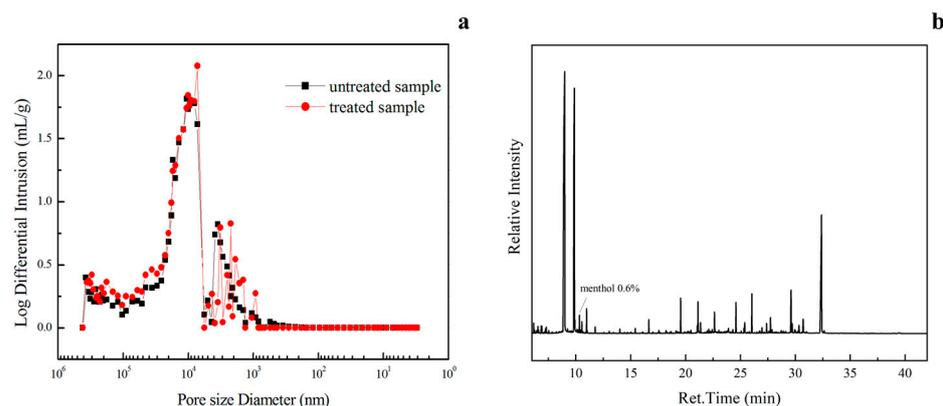
**Figure 6.** (a): Pore size distribution of wood samples (MIP); (b): residual amount of menthol after 10 days (GC-MS).
