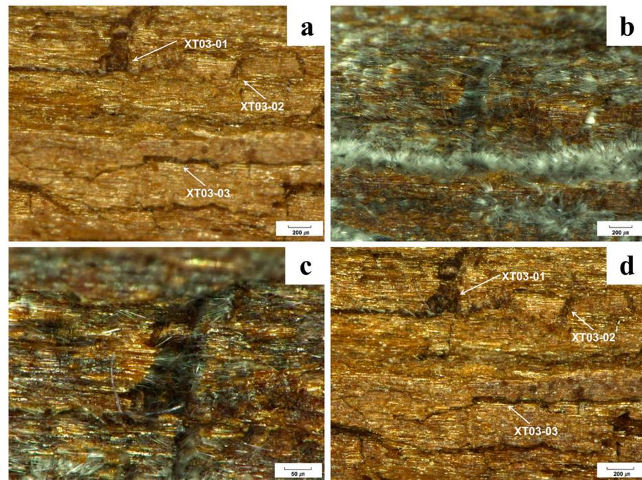
**Figure 4.** Micrographs of sample XT03 during the menthol treatment. (a): Untreated surface (50 $\times$ ), (b): 5 min after menthol treatment, newly grown menthol whiskers appeared (50 $\times$ ), (c): higher magnification of menthol crystals in wood fissures (200 $\times$ ), (d): 10 days after menthol treatment, no visible menthol was observed (50 $\times$ ).
